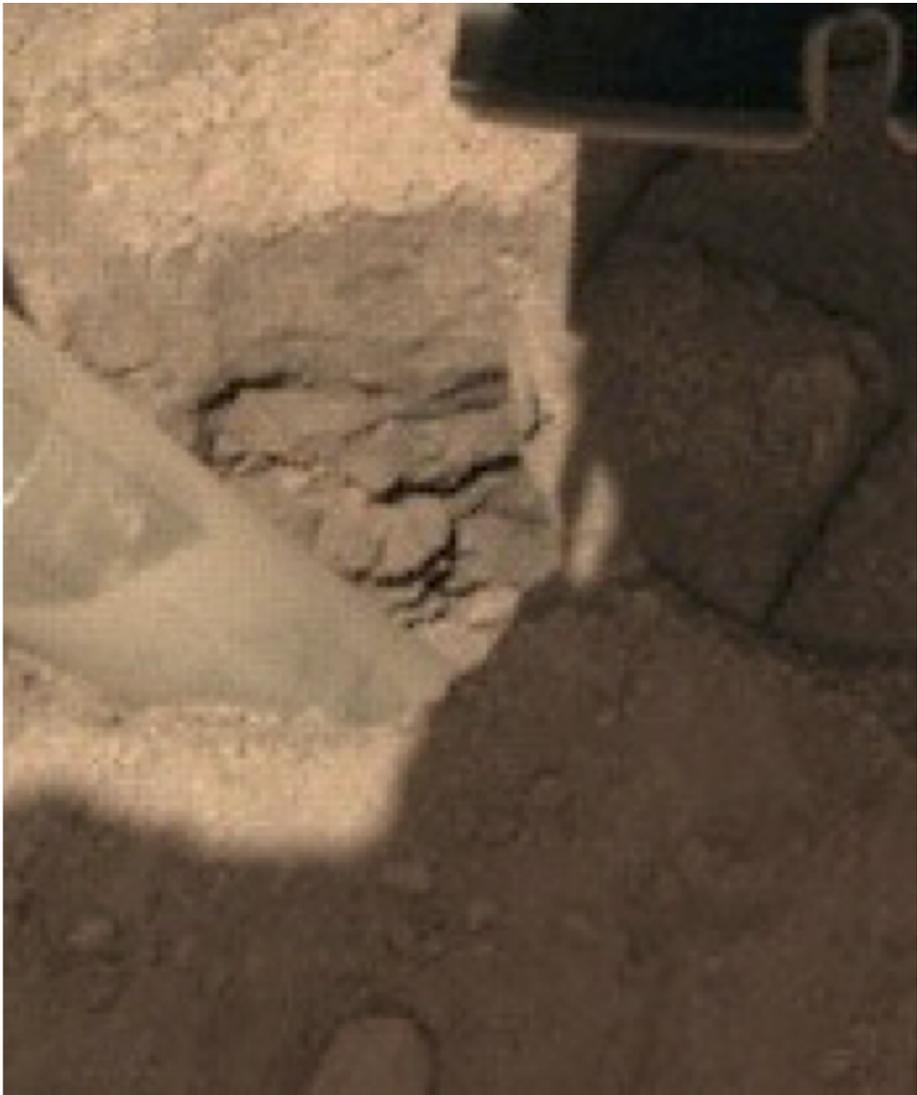
**Fig. 10** Image of the hole created by the HP<sup>3</sup> mole showing the almost vertical southerly wall of the pit and resistant layers in it. These layers have steep edges and overhangs indicating cohesion in the soil. Small rocks appear cemented in a fine-grained matrix, similar to the pits beneath the lander. Mole is in the foreground angled  $\sim 15^\circ$  towards the right
