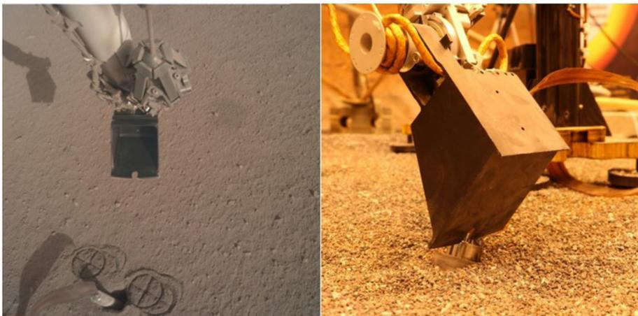
**Fig. 4** The IDA scoop. In the left image, the scoop is shown above the HP<sup>3</sup> mole in this IDC image. The front blade is visible. The grapple is seen stowed to the side of the IDA forearm. In the right image, the scoop in the Earth-based testbed is shown in an “inclined push” configuration on the testbed mole back cap. The dull blade on the outside back of the scoop is visible
