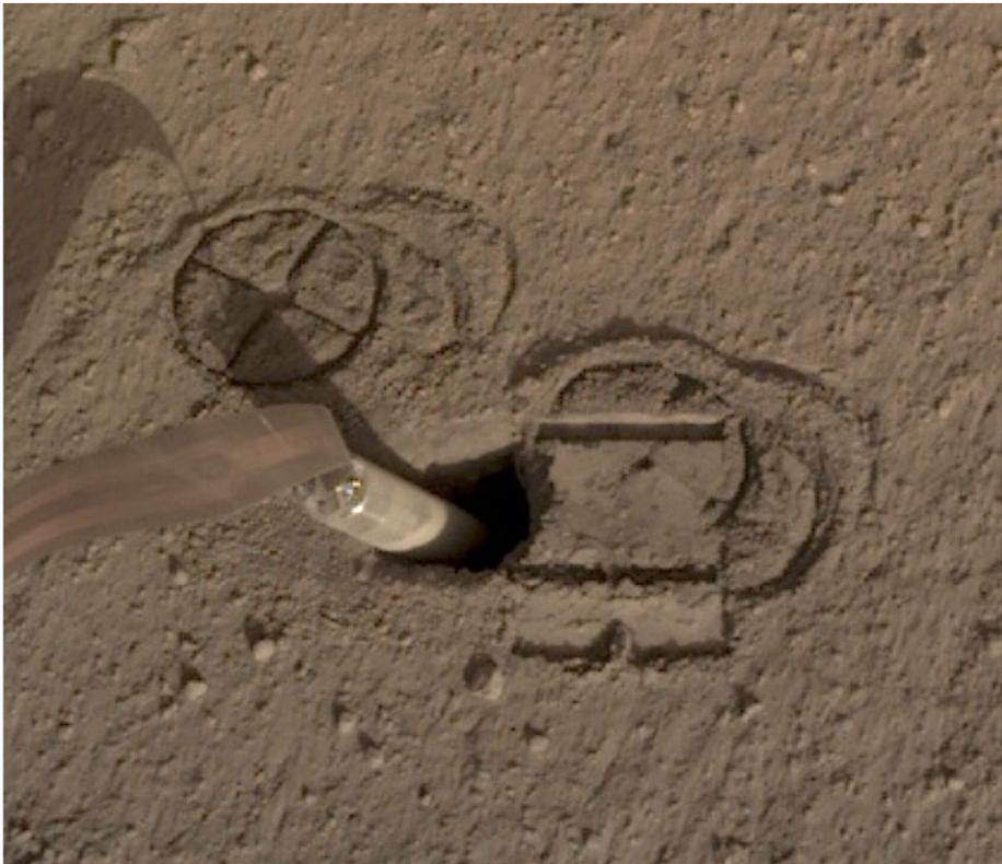
**Fig. 11** Image of mole hole and surface after interactions with the HP<sup>3</sup> SSA feet and scoop. Circular cross patterns are imprints of the HP<sup>3</sup> SSA feet in the soil. Smooth, reflective rectangular surface is where the flat base of the scoop (7.1 cm wide) was pressed against the soil, causing a 5–10 mm indentation. Horizontal troughs near the top and bottom of the scoop imprint are where the front and back blades of the scoop (Fig. 4) penetrated into the soil
