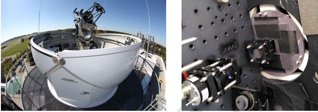
Figure 2. Telescope and dome of Optical Ground Station Oberpfaffenhofen (left). Optical backplane with power sensor installed (right). Image credit: DLR.
