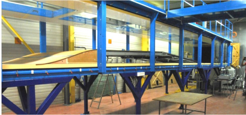
Fig. 5.1: The LML boundary layer wind tunnel with the ramp model (Cuvier et al. (2017))
