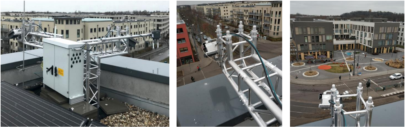
Figure 6: LTSA server with RSU (left) and video cameras (middle, right) in living lab 2
