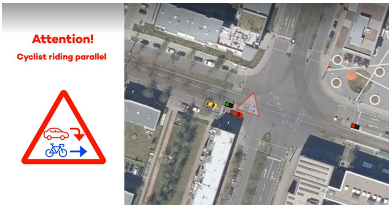
Figure 4: Warning in case of a critical situation between a cyclist (going straight) and a turning vehicle
