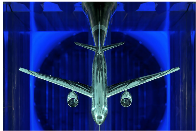
Fig. 2 XRF1 wind tunnel with UHBR through flow nacelles in the ETW test section during the MK2A test entry
