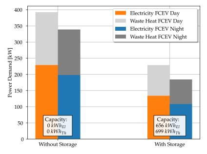
**Figure 4.** Power demand in the neighbourhood, with and without storage capacities. The blue bars show the required electrical power in the period from 7:00 to 19:00. The orange bars show the necessary electrical power in the period from 19:00 to 7:00. The grey bars above show the waste heat from the FCEVs utilised in addition to the electrical power supplied.
