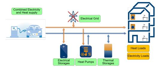
**Figure 2.** Representation of the relevant model elements: fixed load profiles (orange boxes) and variable power flows to be determined (green boxes). The optimal capacity of the electrical and thermal storage capacity is also to be determined by the solver. As a period with low renewable energy being available is considered, no electricity is available from the grid. The model should therefore avoid the draw of electrical power from the grid.
