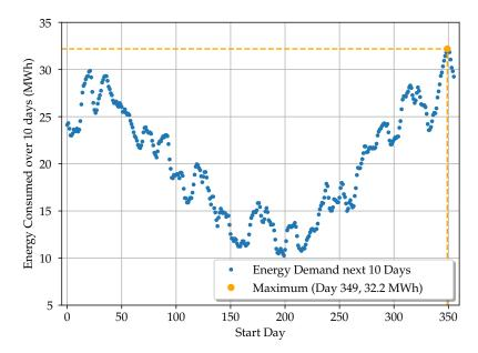
**Figure 1.** Energy consumed in the neighbourhood under consideration in MWh over a period starting at 0:00 on the start day and ending after ten days respectively 240 hours at 23:59 (blue dots). The maximum demand of 32.2 MWh on day 349 is shown in yellow (dashed).
