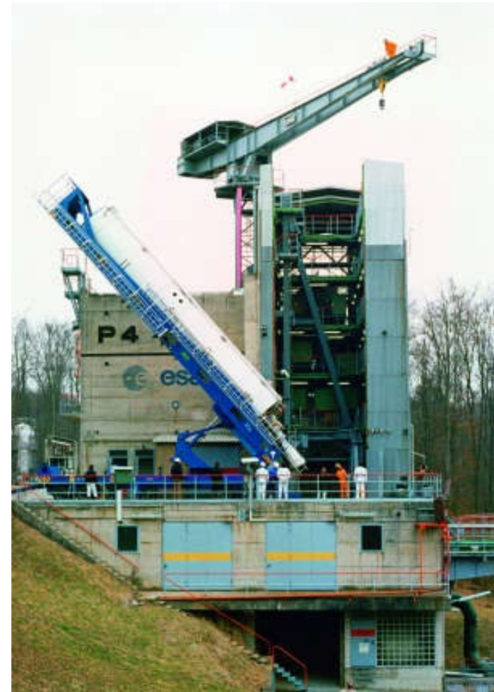
Right: Integration of the PAL booster of Ariane 4 at P4.1
