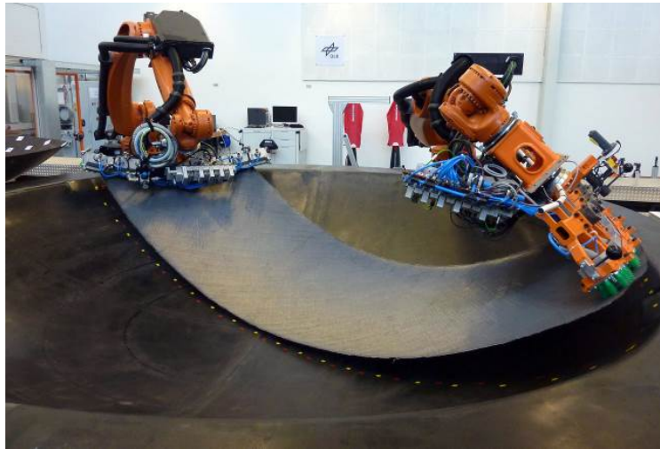
Figure 1: First handling test of large cut-pieces with cooperating robots [1]
