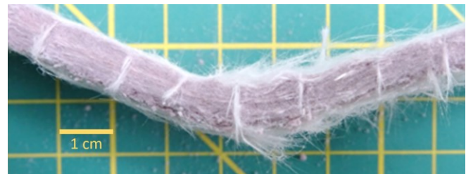
Figure 7 Pyrogel XTE cross section after a bend test
