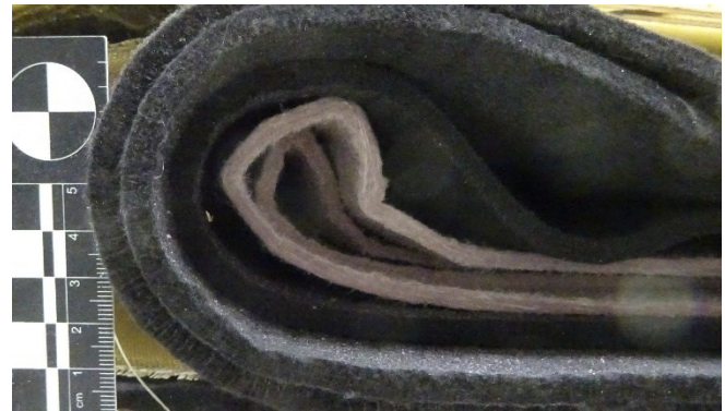
Figure 13 Layup bend test of 3 Sigratherm GFA5 layers and 2 Pyrogel XTE layers
