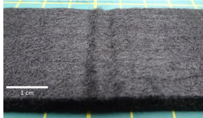
Figure 6 Sigratherm GFA5 surface after bend test
