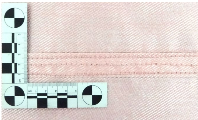
Figure 11 Nextel 440 BF-20 double-felled sewn seam
