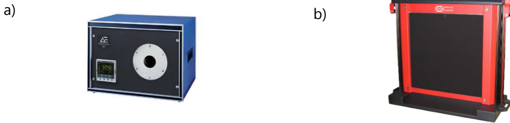
Figure 1.32: Example of reference blackbodies for temperature calibration. a) Mikron M305 cavity blackbody [176]. b) ECN100 extended area blackbody [177].
