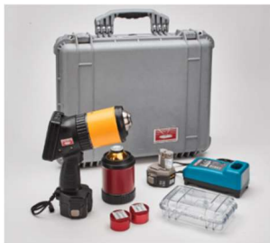
Figure 1.26: Surface Optics Corporation 410-Vis-IR portable instrument. a) Instrumentation, including portable unit, measurement heads and reference calibration coupons. b) Integrating sphere. The red arrow is the illuminating beam. The purple arrow is the reflected beam, green arrows correspond to scattered light.
