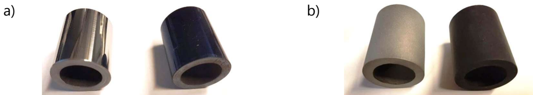
Figure 1.20: Pictures of tubular metal substrates (T91) and STACs. a) Polished metal substrate and SSC. b) Sand blasted metal substrate and HSA coating.
