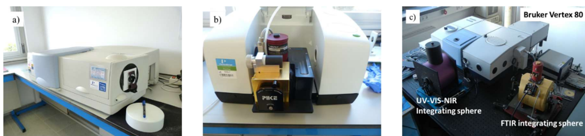
Figure 4.4: Benchtop spectrophotometers a) Perkin Elmer Lambda 1050 b) Perkin Elmer Frontier FTIR with Pike Ltd integrating sphere (upward sample positioning). c) Bruker Vertex 80 with both integrating spheres.
