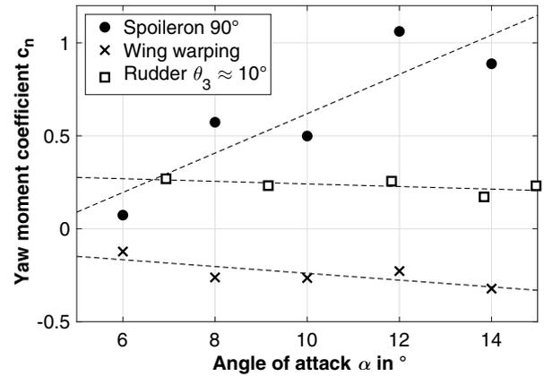
Fig. 12 Yaw moment coefficients due to wing warping and spoileron deflection.
