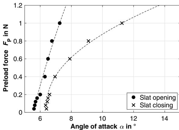
Fig. 10 Preload on leading-edge flap levers; spring rates 2 N/m ( $F_P < 0.2$  N) and 8 N/m ( $F_P > 0.2$  N).
