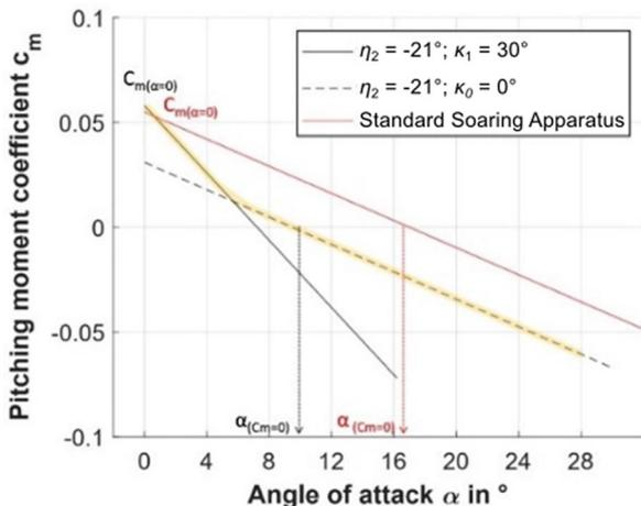
Fig. 7 Linearized pitching moment coefficient around the center of gravity of Standard Soaring Apparatus and Experimental Monoplane for two different settings of the leading-edge flap (at maximum elevator inclination) (partly adapted from [14]).
