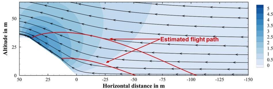
**Fig. 14** Estimated dune cross-section and predicted wind situation at Marina Beach, California, with the vertical wind component shown as contours.
