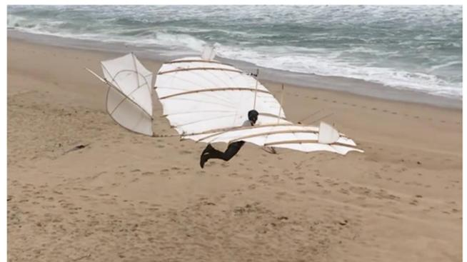
**Fig. 18** A similar flight position, shortly before landing. Andrew Beem is turning the glider to flare by shifting his weight strongly backward.
