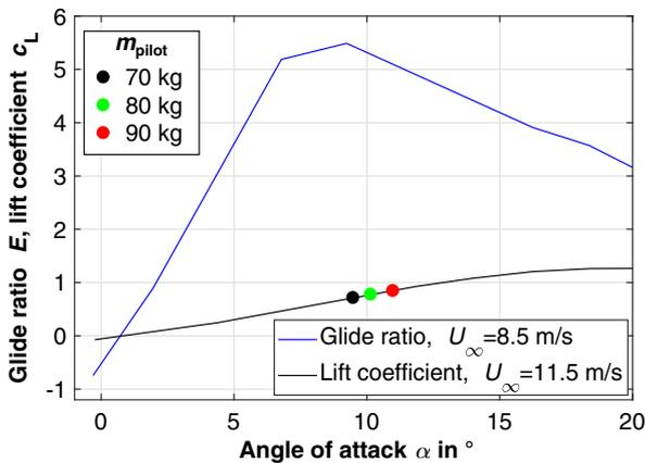
Fig. 6 Glide ratios and lift coefficients of the Experimental Monoplane with closed leading-edge flaps (dots indicate lift coefficients required for various pilot weights at 11.5 m/s).
