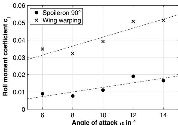
Fig. 11 Roll moment coefficients due to wing warping and spoileron deflection.
