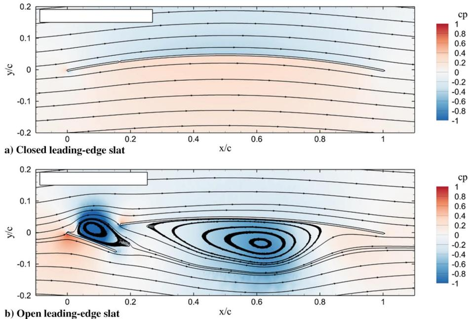
Fig. 9 Color-coded pressure coefficients and streamlines derived from two-dimensional computational fluid dynamics computations for closed (top) and open (bottom) leading-edge flaps.
