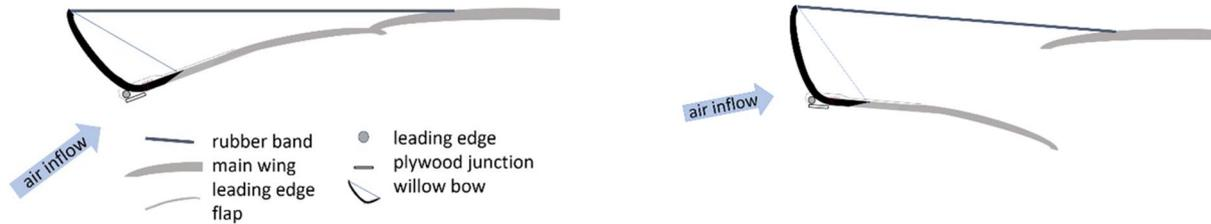
Fig. 8 Closed (left) and open (right) leading-edge flap positions depending on the angle of attack of the incoming flow.
