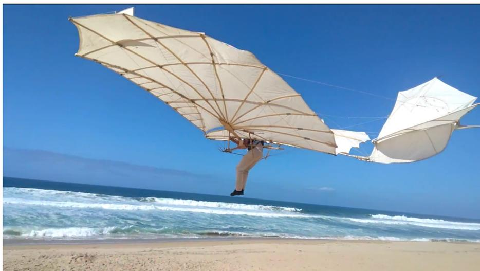
**Fig. 21** Trimmed flights of 72 m maximum distance without tethers; flight distances limited by high tide (Markus Raffel, Marina Beach, California, 2022).
