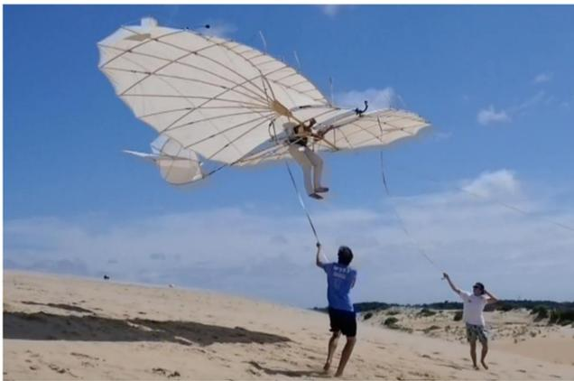
**Fig. 15** Practicing lateral and longitudinal control with limited control authority: tethered flight tests on the Outer Banks 2021.
