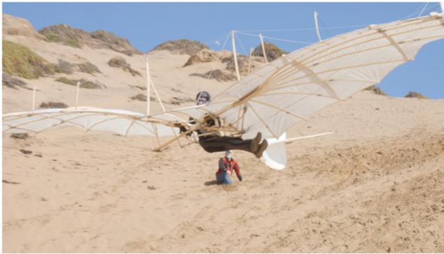
**Fig. 20** Practicing yaw control with the rudder actuated via the hip cradle (Andrew Beem, 2022).
