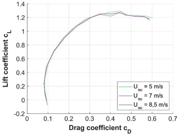
Fig. 5 Lift vs drag of the Experimental Monoplane with closed leading-edge flaps.
