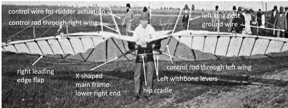
**Fig. 2** Paul Beylich in the Experimental Monoplane with automatic balancing.” Hip cradle, control levers, and rods transferring the control input to the strings above the wings can clearly be seen (adapted from the photograph by R. Neuhaus, 1895, © Archiv Otto-Lilienthal-Museum).
