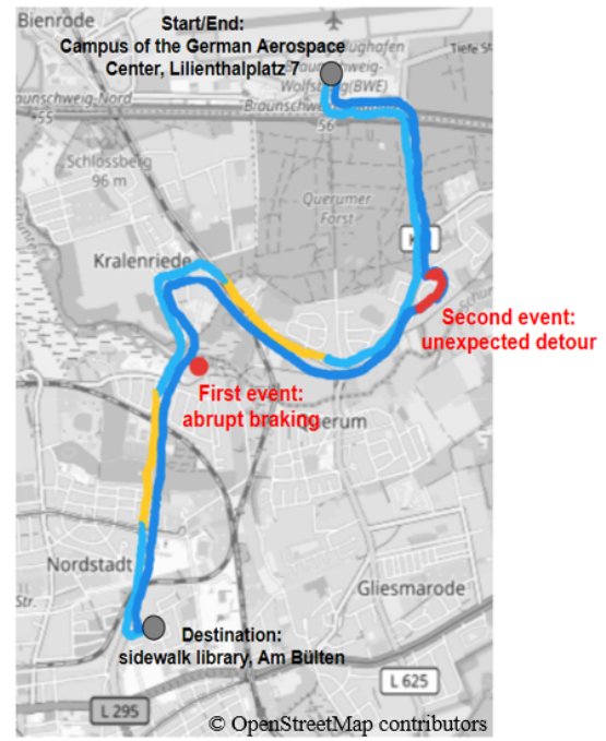
Fig. 1. Driving route of the vehicle. Light blue and orange lines indicate the forward run. The orange sections mark the baseline routes for the analyses of the physiological data. The dark blue line indicates the return path. Two events occurred, which are marked in red.
