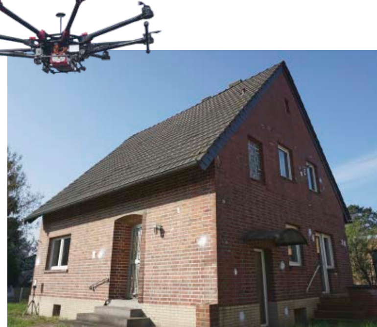
A small drone surveys buildings in terms of their geometric, physical, energetic and functional properties.
