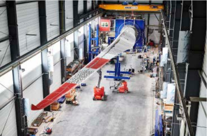
Testing the vibration and load behaviour of the rotor blades
