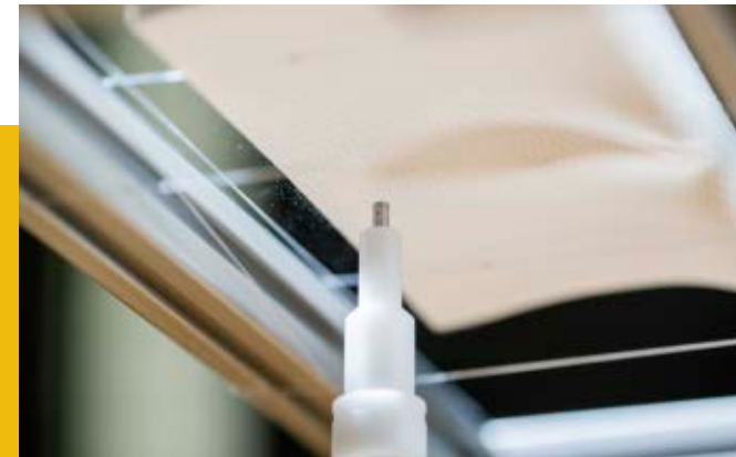
A projectile taps the component and causes it to vibrate
