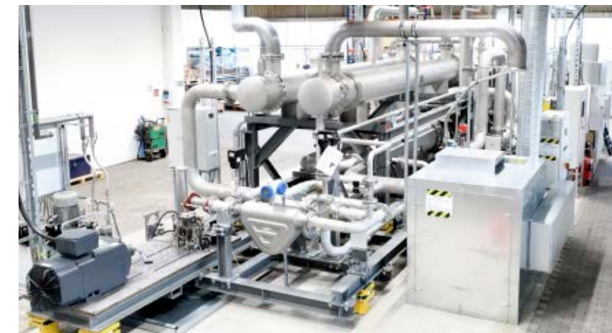
This prototype of a special high-temperature heat pump called CoBra is located at the DLR Institute of Low-Carbon Industrial Processes in Cottbus. The system can provide heating and cooling for industrial processes on a demonstration scale.
