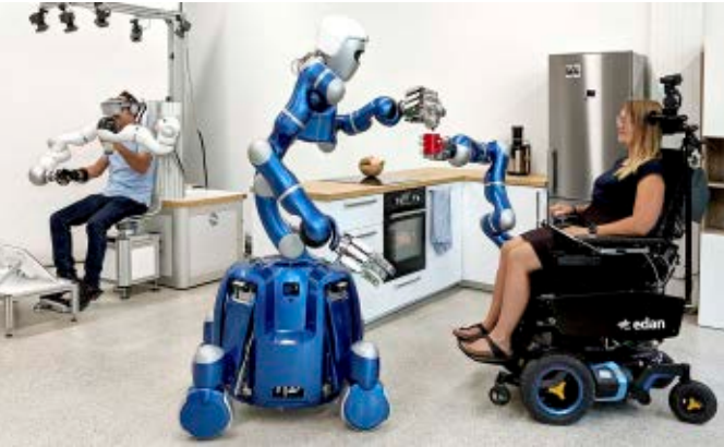
Several systems are being tested in the project: on the left, a haptic input station with two lightweight arms (HUG); in the centre, the humanoid, two-armed mobile home assistance robot Rollin’ Justin; and on the right EDAN, a wheelchair with a lightweight robotic arm and a hand.
