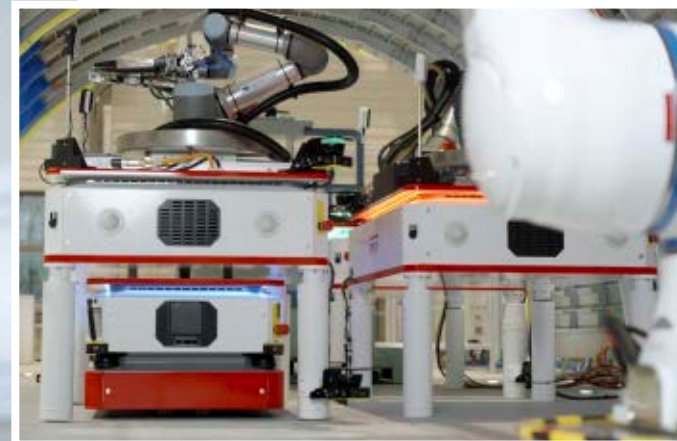
Mobile transport units bring the robots to their workstations. They are equipped with sensors that register movements. If a person gets too close to them, they stop until the path is clear.
