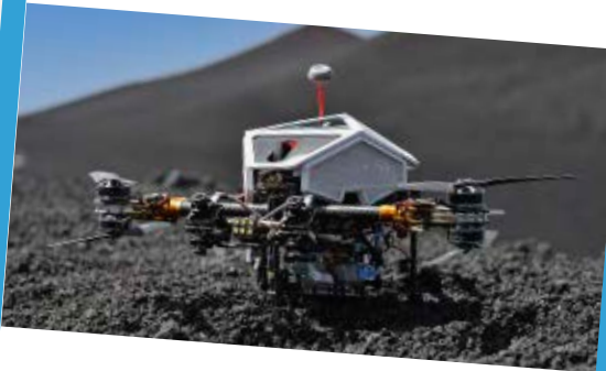
Ardea is a micro aerial vehicle (MAV) equipped with four cameras with ultra-wide-angle lenses that cover a vertical image area of 240 degrees. This allows Ardea to see above and below at the same time, making it much easier to carry out navigation and mapping activities in tight spaces such as caves.
