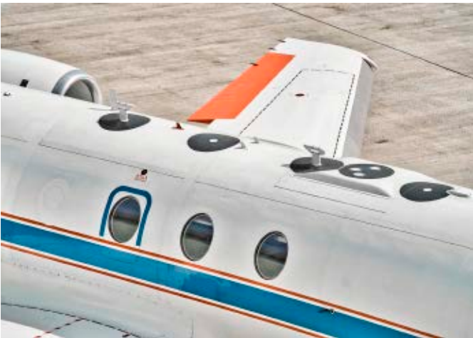
The sensors for laser absorption spectroscopy are located on the rear of DLR's Falcon research aircraft. They investigate how strongly the oxygen molecules in the atmosphere absorb the laser beam between the sensors.
