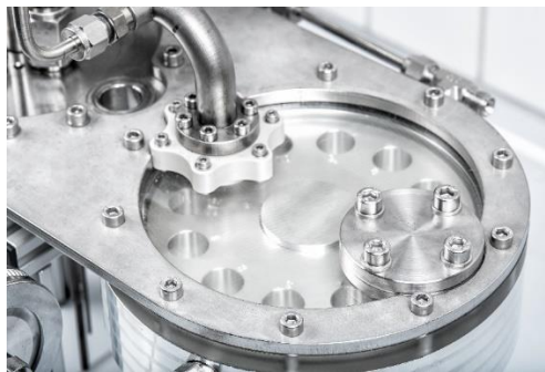
Figure 1 Autosampling system used for sample extraction during long-term experiments with Solar Salt at high temperatures.
