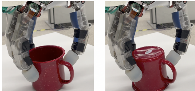
Fig. 1. Purely tactile in-hand pose estimation with the DLR-Hand II [2], where contacts with the fingers are detected based on the hand's torque sensors (see Section IV for details). Many everyday objects, like the mug shown here, exhibit apparent symmetries ; the same tactile measurement can be compatible with multiple poses, often infinitely many. A state estimator addressing this problem should be able to represent the rich, multimodal belief distributions that arise in these settings.
