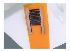
Figure 8. Fabrication of porous LIG -electrodes based in-plane micro-supercapacitor (IMSC).
