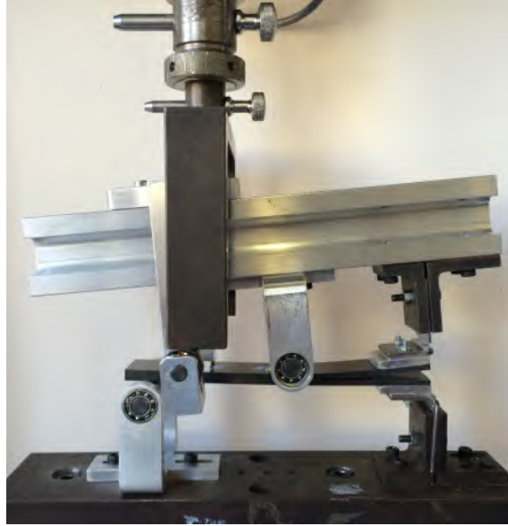
Figure 5.9: MMB specimen inside fixture according to ASTM D6671
