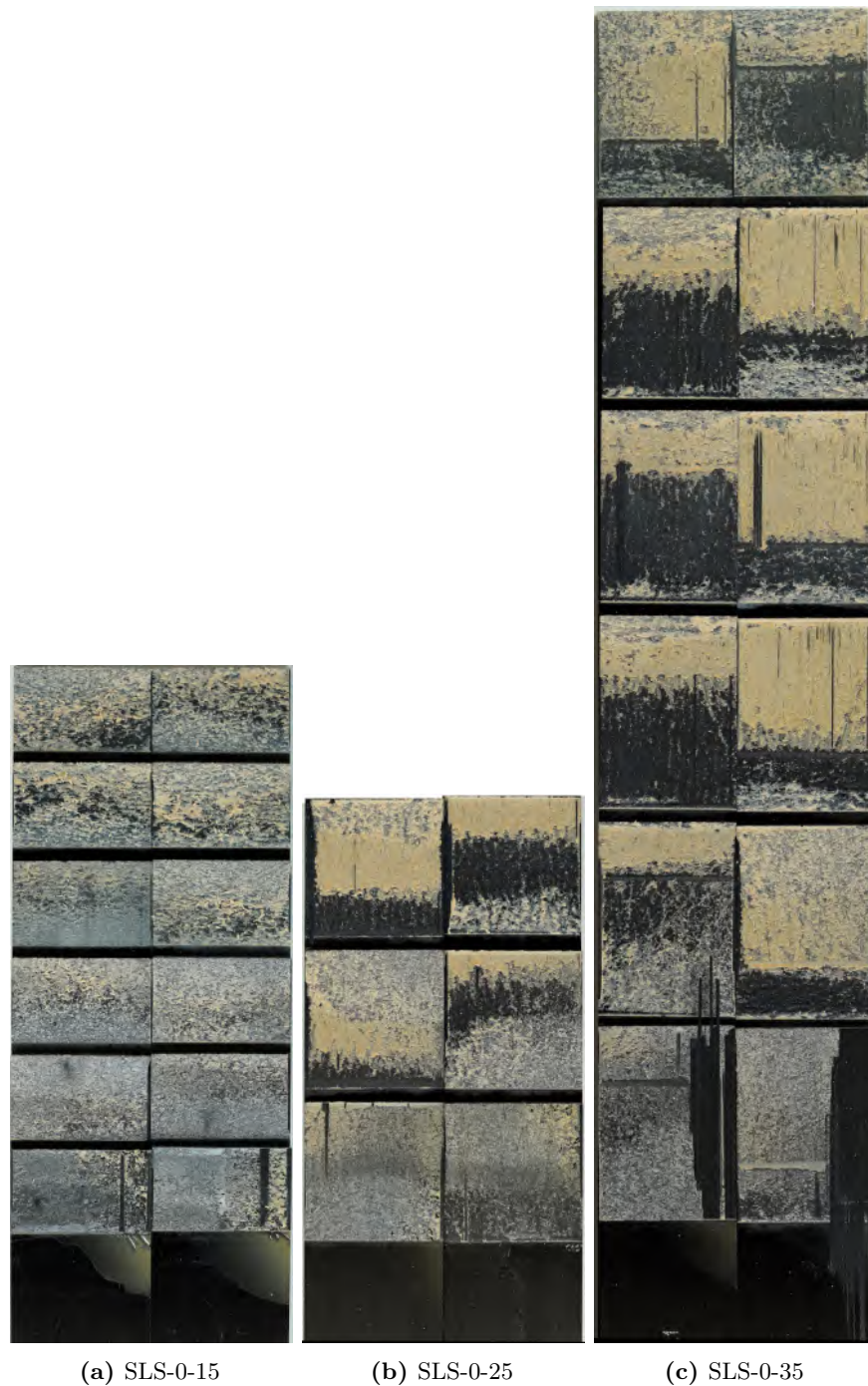
Figure I.1: Cohesive fracture patterns of SLS-0 specimens
