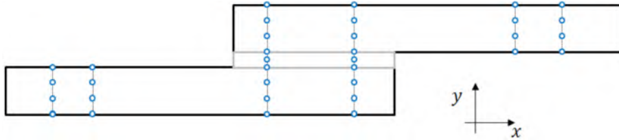
Figure 8.7: Front view for coupling of displacement u_z applied on the nodes with the same x -coordinate belonging to the vertical lines on the edge adopted from [300].
