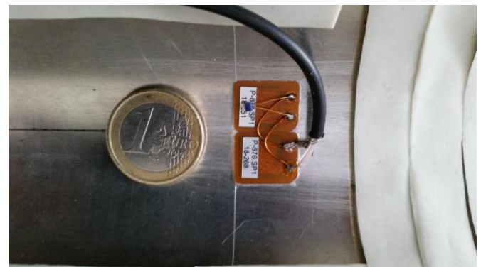
Figure 8: Transmitter piezoelectric patches compared to Euro coin
