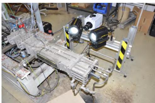
(a) Atmospheric combustion chamber set-up with optical diagnostic at M11.3
