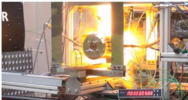
(b) Flame flashback and destruction of feeding line during initial testing with premixed, liquid HyNOx
