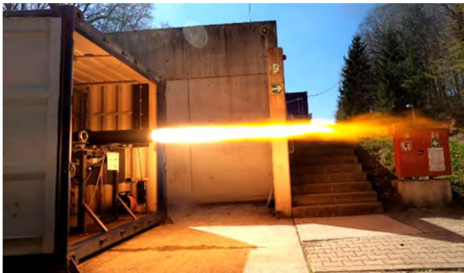
(b) Firing test of the 10 kN LOX/Paraffin-based hybrid engine at M11.5 [33]
