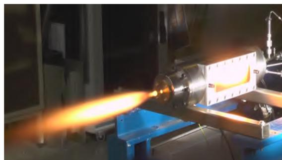
(b) Pressurized combustion chamber with optical access at M11.3
