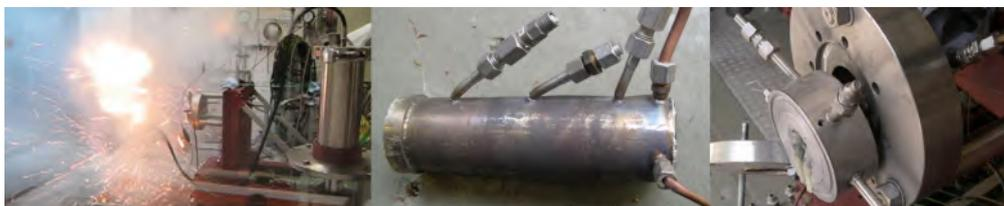
Figure 18: Deflagration event and its aftermath in a 2009 hot test with an early nitromethane-based gel at the M11.4 test bench
