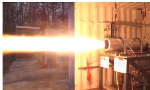
(b) Firing test of 10 kN  $N_2O$ /Paraffin-based hybrid engine at M11.5
