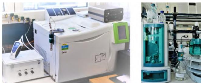
Figure 2: left: Gas chromatograph (Perkin Elmer); right: ion chromatograph (Metrohm)
