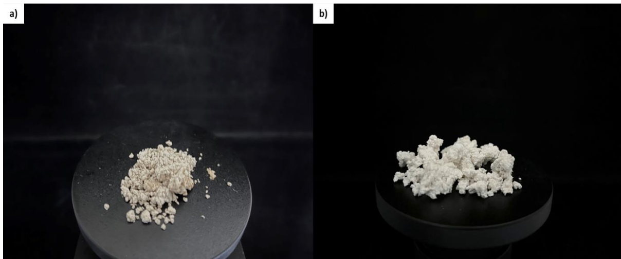
Figure 22: Dried alkalization product (left) and dried cellulose after bleaching (right)
