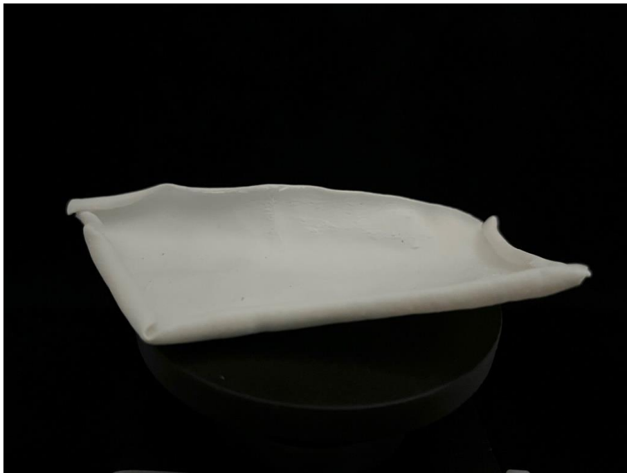
Figure 25: Cellulose aerogel sheet.
