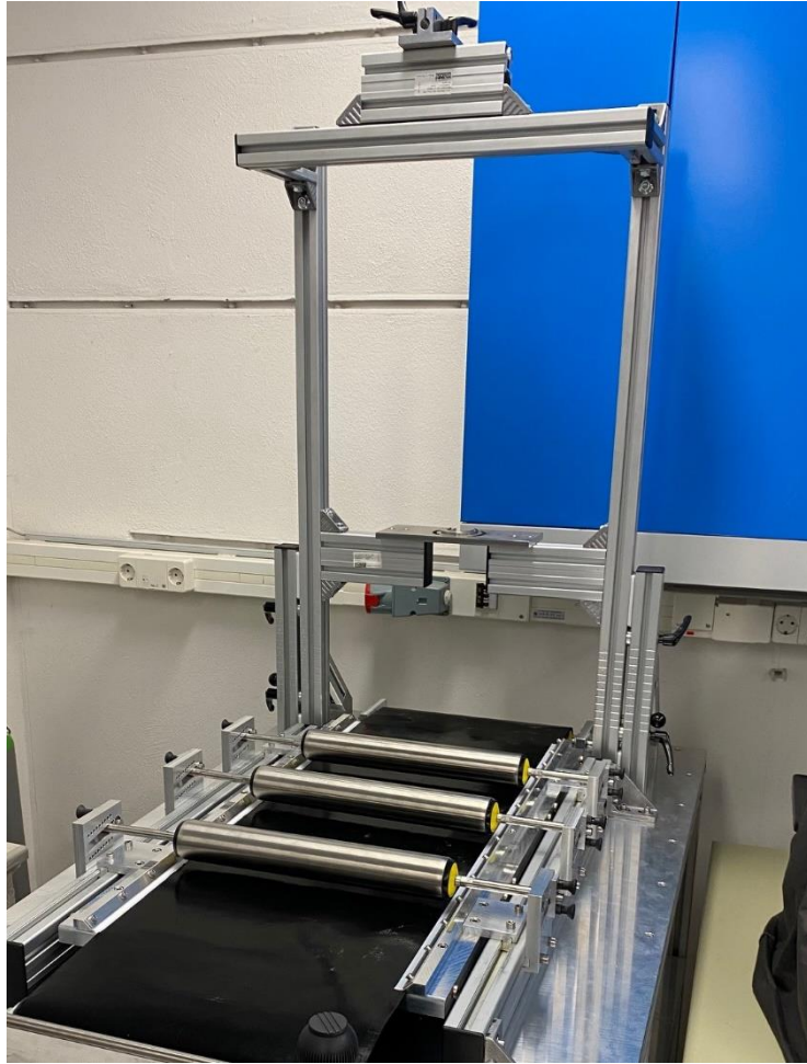
Figure 24: Setup CaProLi for sheet production.
