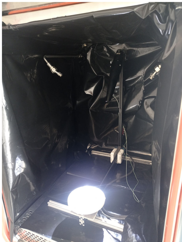
FIGURE 5 Setup for testing the temperature dependence of the lamps in a Vötsch-ATLAS SC340_MH climate chamber
