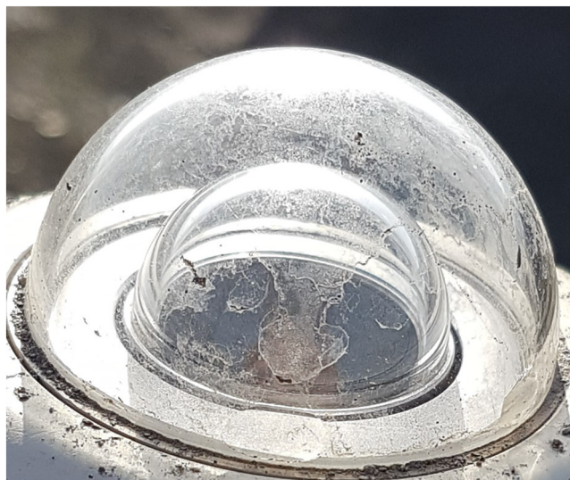
FIGURE 14 Pyranometer dome after artificial soiling on 19 January
