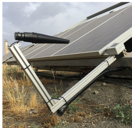
FIGURE 1 Soiling loss measurement systems for a pyranometer installed on a fixed structure (left) and for a reference cell/PV (right)
