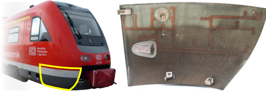
Figure 6 Lightweight structural component with integrated SHM system in a railway field trail, project faWaSiS (Trampe et al. 2021)
