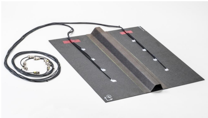
Figure 5 Specimen plate with omega stringer and SHM sensors, project DEMETER (Moix Bonet et al. 2018)
