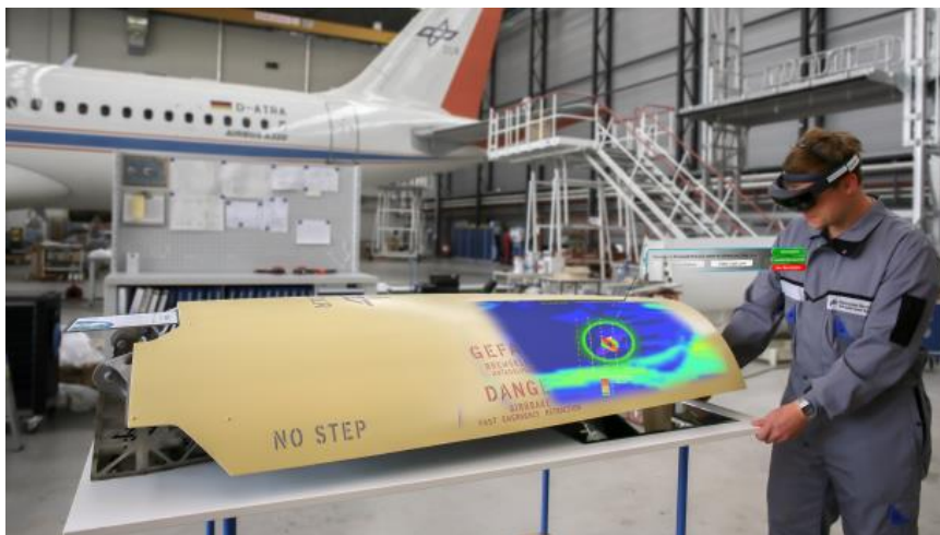
Figure 8 Demonstration of a SHM system combined with structural analyses displayed in augmented reality glasses on the structure of a Typhoon Eurofighter Airbrake (Kaps et al. 10/1/2019)
