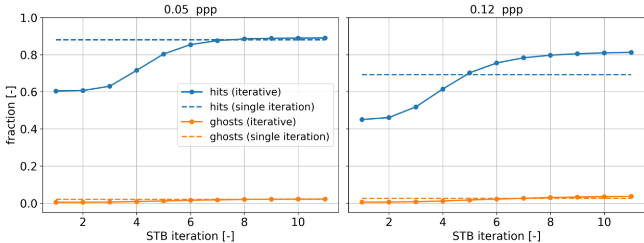
Figure 3. Fraction of reconstructed tracks from TP-STB with respect to the number of tracks from the reference TR-STB solution for both particle image densities. The fraction of correctly reconstructed tracks ( hits in blue) and of ghost tracks ( ghosts in orange) are shown for a single iteration (dotted line) and for the complete iterative TP-STB strategy.
