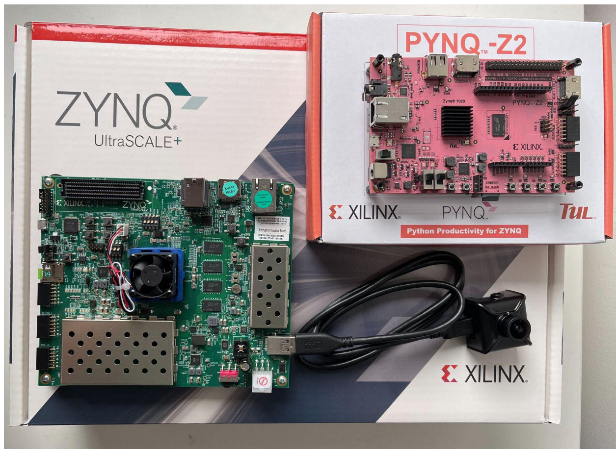
Figure 46. On the left side the ZCU104 evaluation board, and on the right top, the PYNQ-Z2 evaluation board. [Source: Author]
