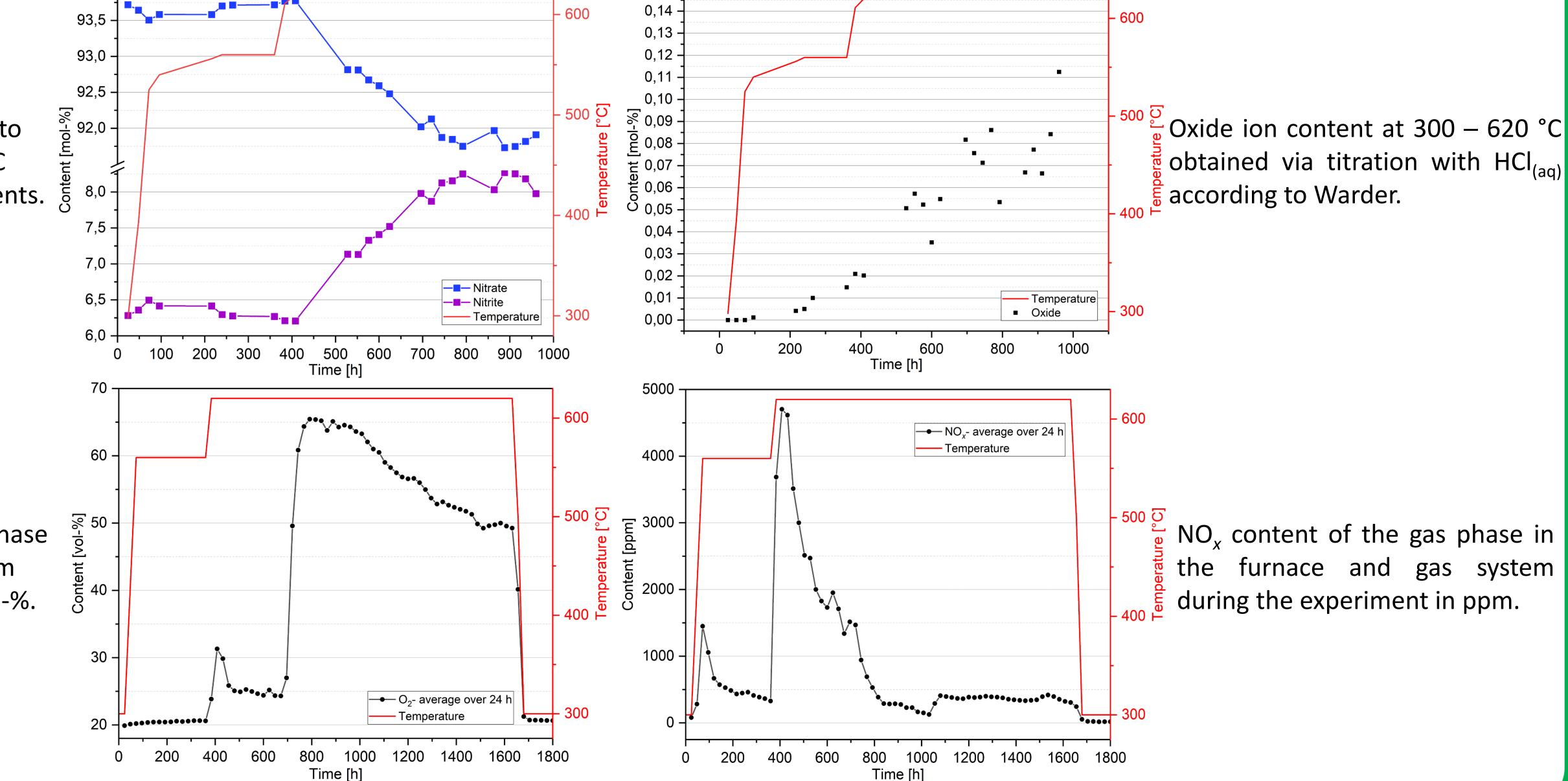
Oxygen content of the gas phase in the furnace and gas system during the experiment in vol-%.
