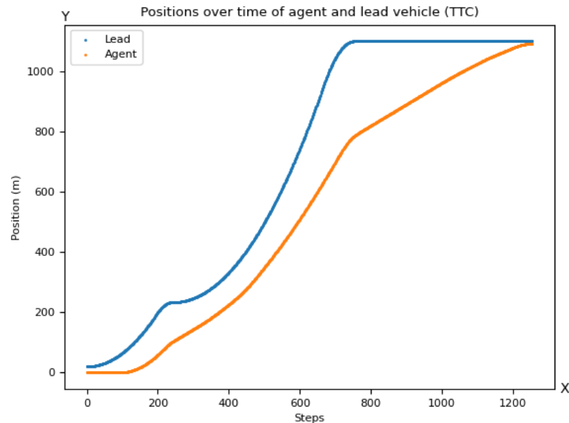
Figure 12. Positions over time of the agent (orange) after 10 million steps of training with time to collision reward vs. leading vehicle (blue).
