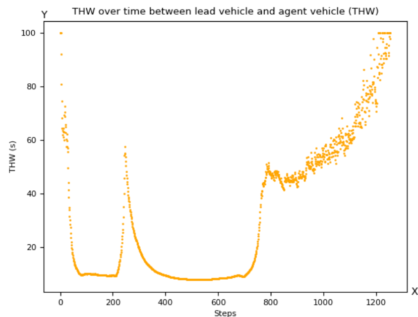
Figure 9. Time headway over time for the time headway metric reward.
