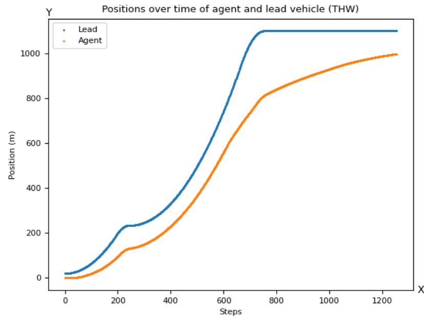
Figure 8. Positions over time of the agent (orange) after 10 million steps of training with time headway reward vs. leading vehicle (blue).
