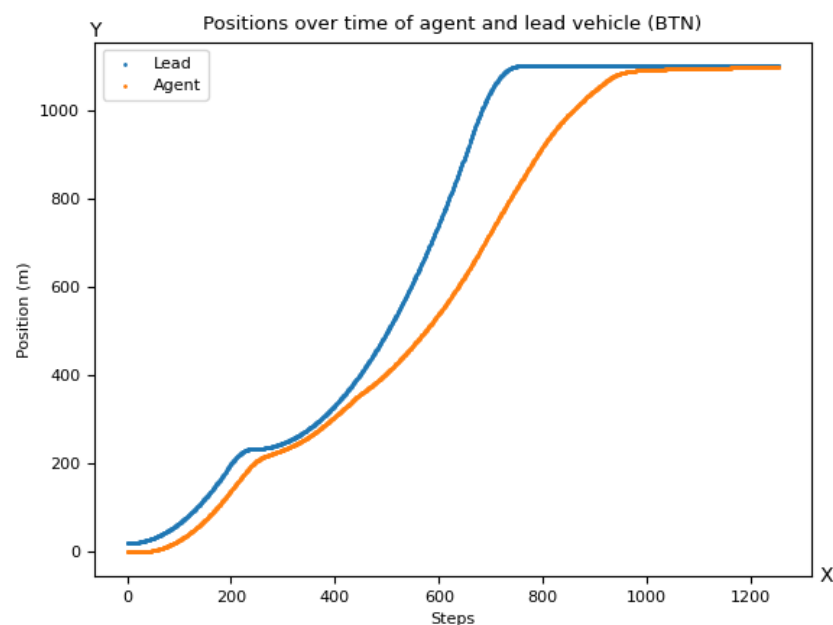
Figure 24. Positions over time of the agent (orange) after 10 million steps of training with the brake threat number reward vs. leading vehicle (blue).
