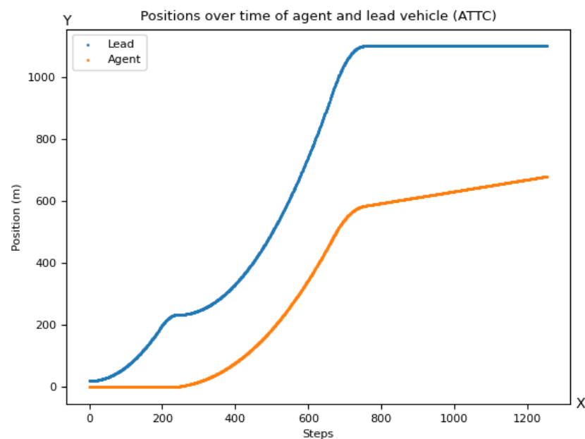
Figure 20. Positions over time of the agent (orange) after 10 million steps of training with the ATTC reward vs. leading vehicle (blue).
