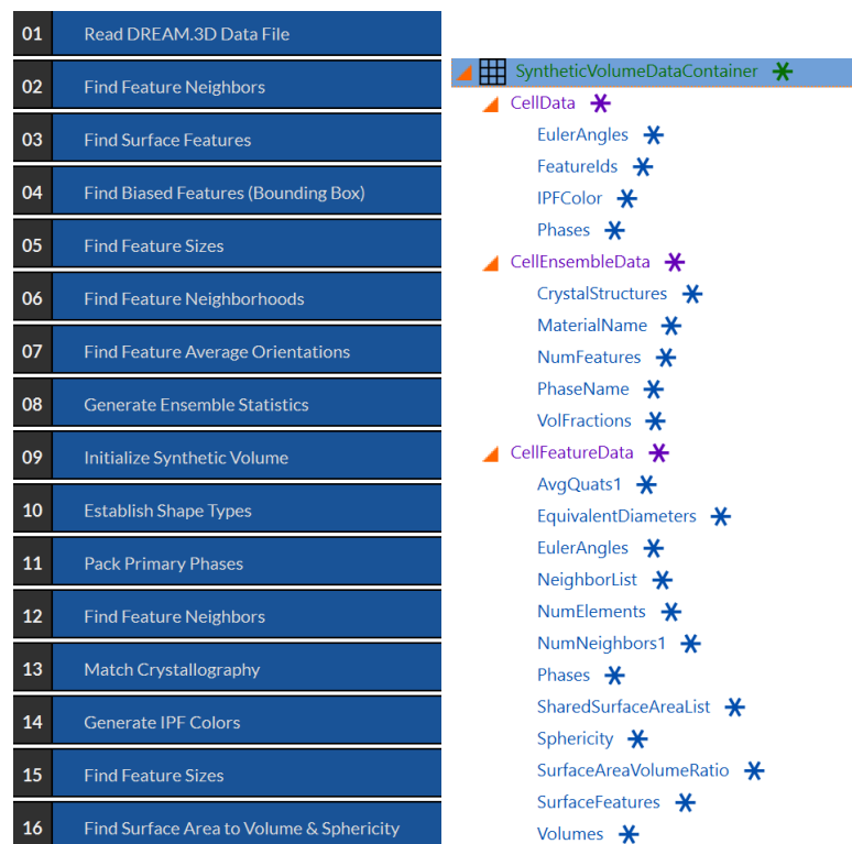
Figure 2.3: Pipeline to generate equivalent 3D volume elements from 2D EBSD Image and the corresponding Data Structure (Synthetic Data Volume)*
