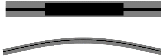
Figure 6: Top: Optimal design of the first bending mode from top view. Black color indicates added core and face layers. Bottom: Mode shape of first bending mode.
