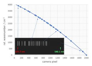
**Figure 2:** Spectral calibration of the BBM with a Ne lamp in the range of 0 to 4000 cm<sup>-1</sup>. Inset: Raw detector image with the individual slit images.
