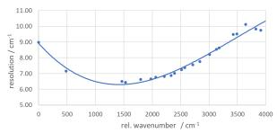
Figure 3: Spectral resolution across the spectral range.
