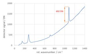
**Figure 4:** Raman spectrum of calcite. The 1086 cm<sup>-1</sup> line achieves an SNR of > 800 (exposure time: 60s).
