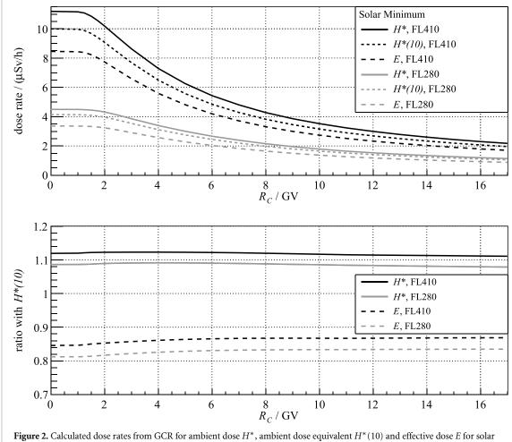
Figure 2. Calculated dose rates from GCR for ambient dose  $H^*$ , ambient dose equivalent  $H^*(10)$  and effective dose E for solar minimum conditions at FL280 and FL410 as a function of cut-off rigidity  $R_C$  (top); corresponding ratio of  $H^*$  and E with  $H^*(10)$  (bottom).
