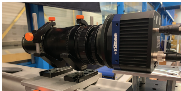
Figure 2. Imaging setup for the present experiment including a 47 MPixel CCD camera and a 250mm-focal-length telephoto lens with extension tube.
