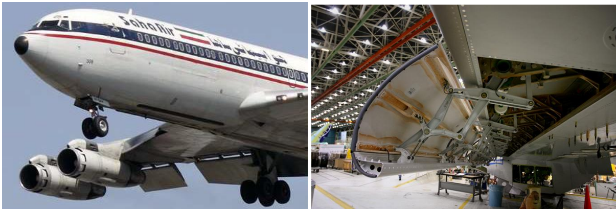
Figure 1: Krueger flaps inboard of a Boeing B707 (left – image obtained from www.wikiwand.com ) and the outboard variable camber Krueger flap of the Boeing B747 (right – image obtained from www.wired.com ) © Jason Paur)
