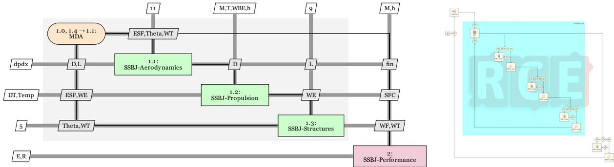
Figure 9. XDSM view (left) and RCE workflow (right) of the collaborative MDAO workflow for analyzing one supersonic business jet configuration, modeled in MDAx.
