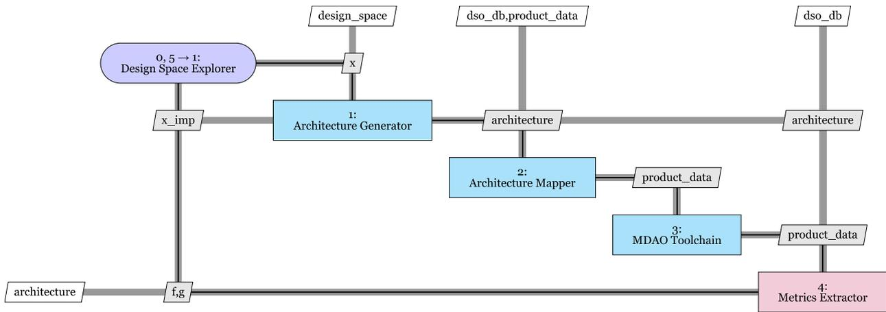
Figure 5. Optimization loop with architecture evaluation: the design space explorer (i.e. optimizer) suggests a design vector ( $x$ ) that is converted into an architecture description. Generated architectures are mapped to a central data schema instance ( $product\_data$ ) using the data schema operation database ( $dso\_db$ ), which is then used to execute the collaborative MDAO toolchain.
