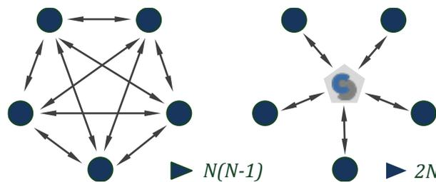
Figure 4. The use of a central data schema like CPACS reduces the number of implemented data interfaces from  $N(N-1)$  to  $2N$ . Reproduced from (Alder, et al., 2020).
