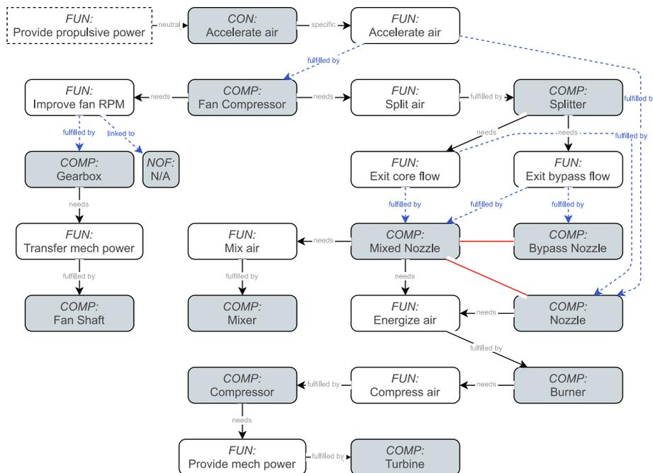
Figure 7. Partial view of a jet engine architecture design space model in ADORE.
