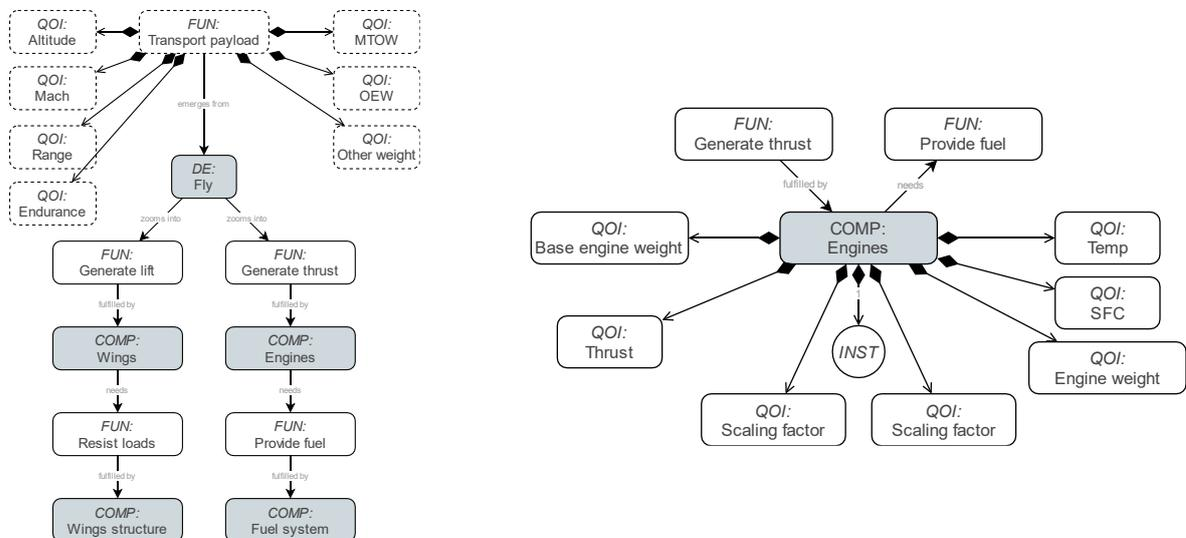
Figure 10. ADORE architecture design space model of the supersonic business jet, showing the system overview on the left, and “Engines” component details view on the right.
