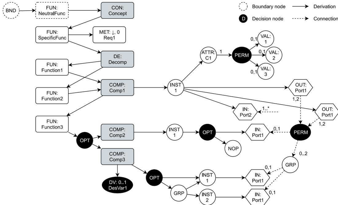
Figure 3. Example Architecture Design Space Graph (ADSG). Directed edges indicate derivation, decision nodes indicate a selection of mutually-exclusive options. Figure reproduced from (Bussemaker, et al., 2020).
