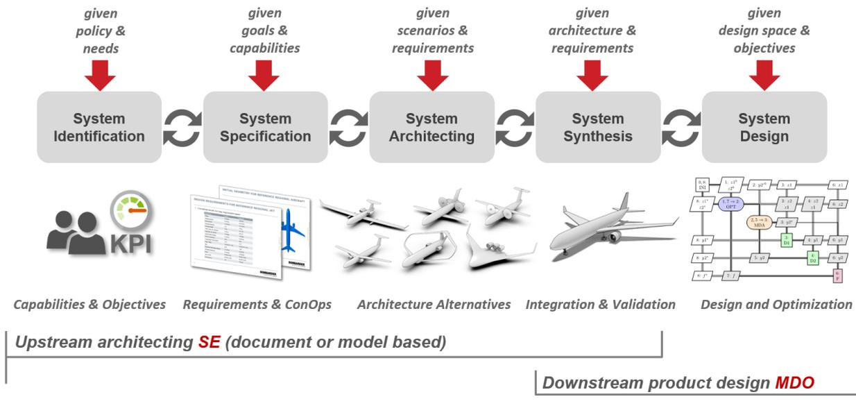
Figure 1. The MBSE framework developed in the AGILE4.0 project, showing the different phases and relation to systems engineering and MDAO. Reproduced from (Ciampa & Nagel, 2021).
