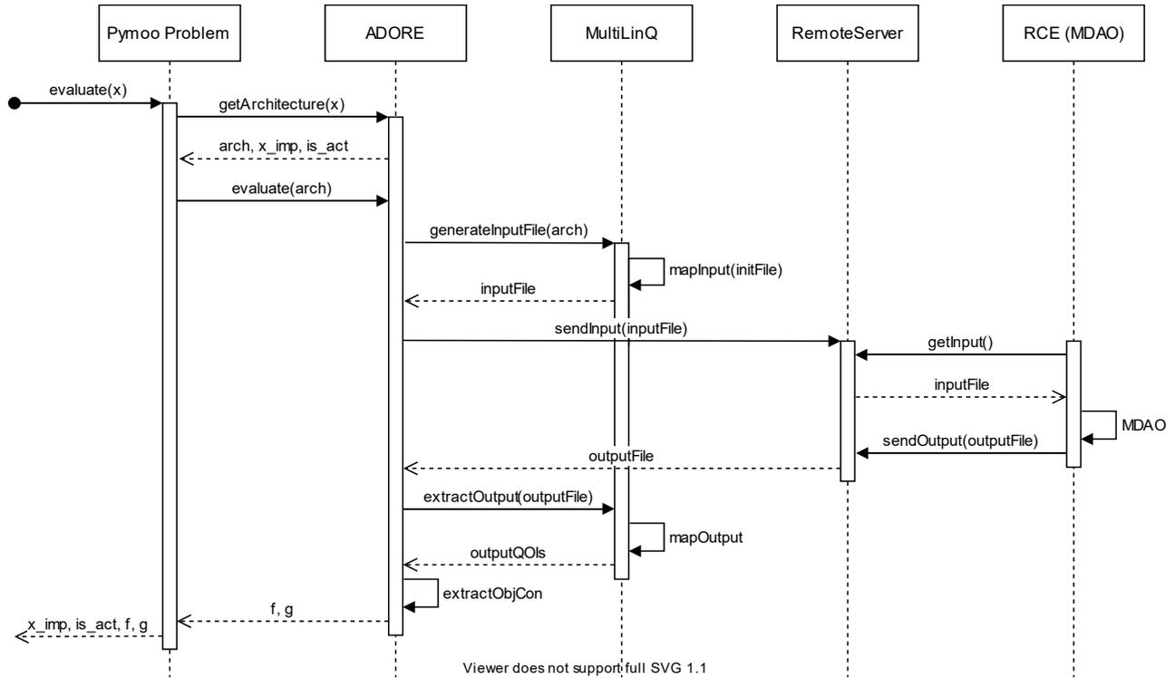
Figure 12. Sequence diagram showing what happens when a design vector ( $x$ ) is evaluated in the optimization loop. The remote server implements the mechanism for sending the input file from ADORE to RCE, where the collaborative MDAO workflow is executed.
