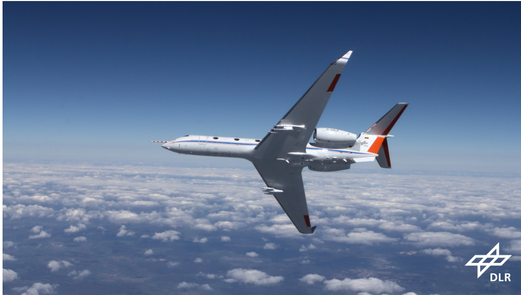
FIGURE 8.7: HALO performing a banked turn. The under-wing stores (PMS carriers) are visible under both wings. Photo credit: DLR.
