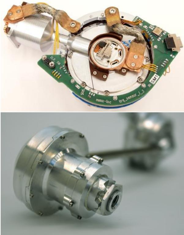
**Figure 3:** The shoulder module (top) and the full locomotion module, consisting of shoulder, leg and wheelhub (wheel not mounted) (bottom)
