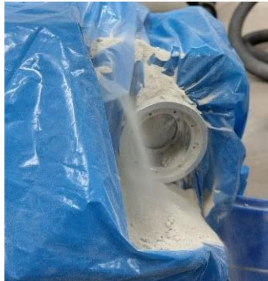
**Figure 8:** Setup of the dust break-in test: The external part of the shoulder sticks out of the protective blue foil and is covered with sand.
