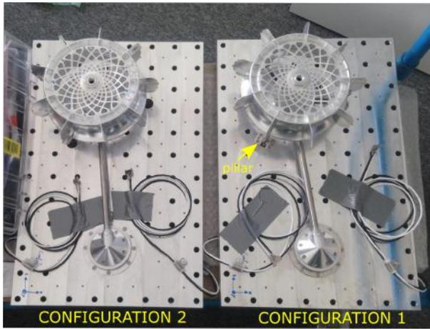
**Figure 7:** Configuration 1 (with pillars) and 2 (without pillars) for shaker test
