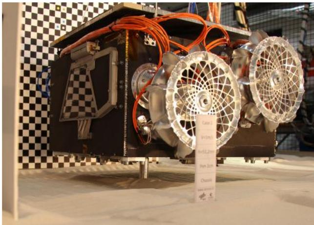
(a) The full rover mockup is dropped onto a target.
