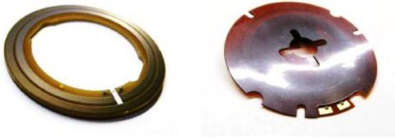
**Figure 16:** FR4-based (left) and Polyimide-based rotational Sensor (right)
