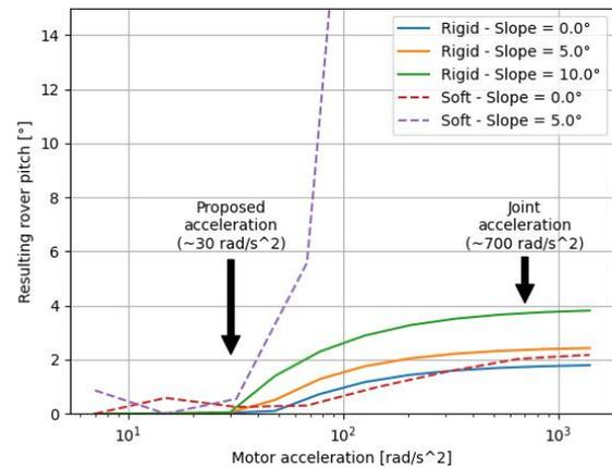
Figure 20: Rover pitch plotted versus the motor acceleration for different slopes on soft and rigid terrain.
