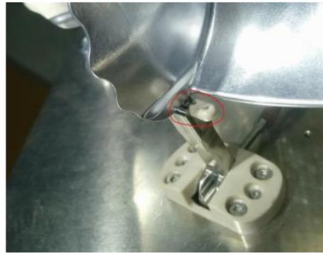
**Figure 5:** The standoff, which supports the wheel to the side, was broken during the drop test.
