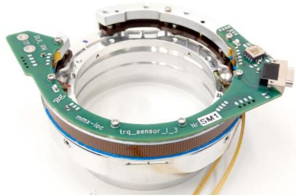
**Figure 17:** Torque-Sensor with PCB and heater
