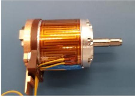
**Figure 10:** One actuator unit consists of the motor, two gear stages and a backshell with three hall sensors. The whole actuator is wrapped with a double-layer heat foil, see section 6.
