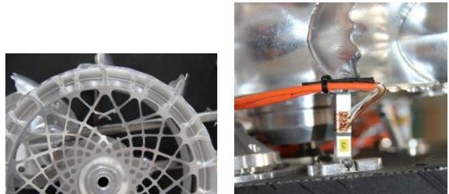
(a) Local damage of the wheel spoke structure without impact on functionality.
