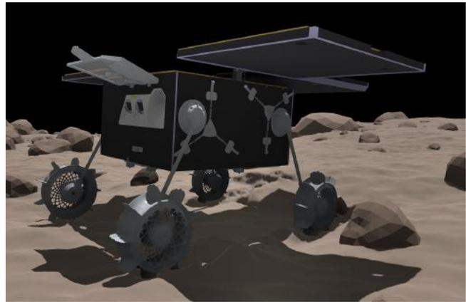
**Figure 1:** Simulation view of the full rover in drive configuration. The LSS components outside the chassis, i.e. the external shoulder side, the legs, wheels and HDRM, can be seen.
