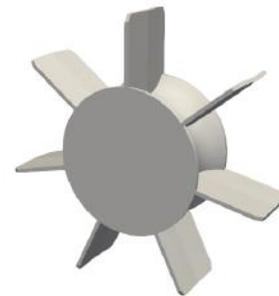
**Figure 12:** Traction-optimized wheel shape for Phobos [7]
