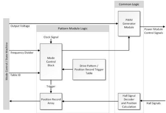
Figure 19: "Pattern" mode design architecture.
