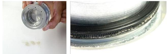
**Figure 9:** Inspection of the hardware after the dust break-in test. A small number of particles reached the outside of the PTFE seal.
