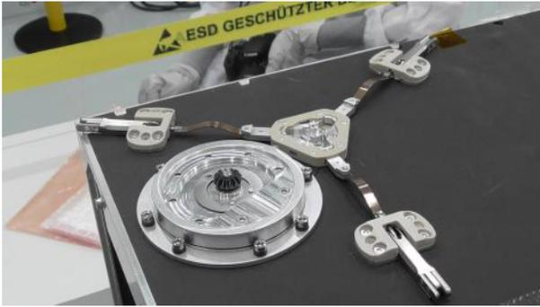
**Figure 11:** HDRM unit (EM) in released state consisting of three pillars and central cone interface during Structural Model integration
