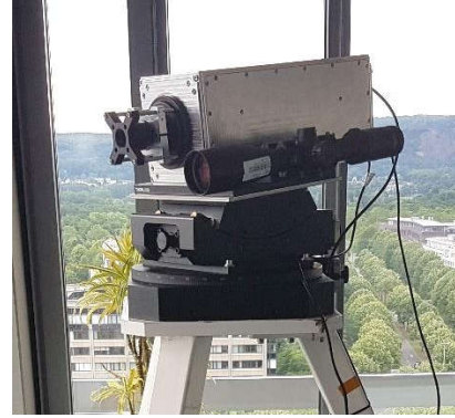
Figure 5: Picture of Alice terminal mounted on the CPA (goniometer and rotation stage) and a tripod with external rifle scope.
