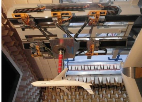
Figure 2: The Model Positioning Mechanism (MPM) in the DNW-NWB, supporting the DLR F12 model
