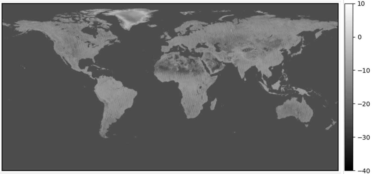
**Figure 2** X-band global backscatter map without gaps, i.e., after missing values interpolation. Backscatter mean value in dB referred to HH polarization and to  $40^\circ$  output reference incidence angle.
