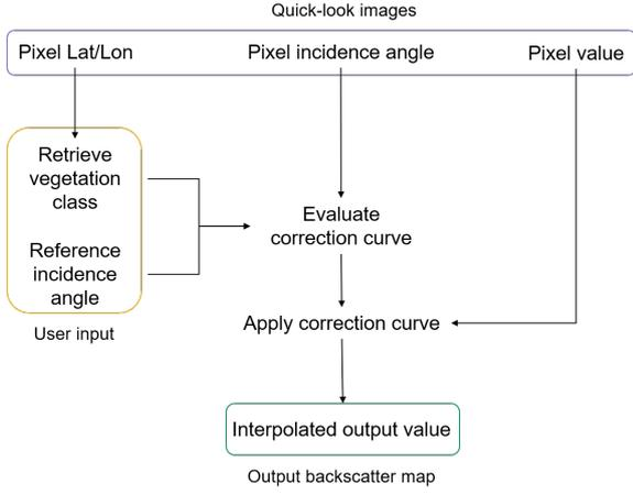
**Figure 1** Algorithm flowchart. The output backscatter map is referred to a precise reference incidence angle.
