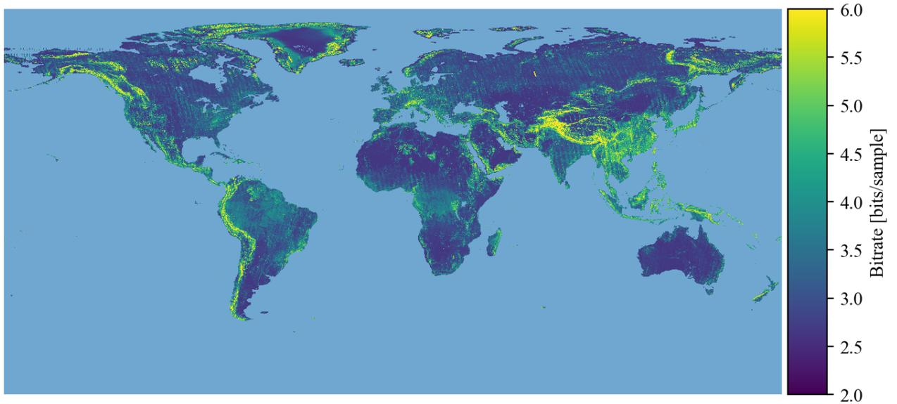
**Figure 3** Global bitrate map resulting from a requirement on the interferometric phase error of  $\sigma_{\Delta\varphi_q} = 5^\circ$ .
