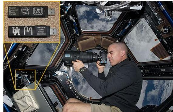
Fig. 2 Space qualified miniaturized Timepix detector (in both yellow boxes) mounted in the cupola of the ISS. These detectors on ESA Proba V satellite are used for years to monitor the dangerous particle radiation in the South Atlantic Anomaly (SAA).
