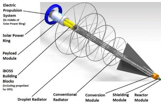
Fig. 1 The 1MW electric class reactor plus all non-nuclear subsystems of the futuristic designed INPPS flagship are displayed.
