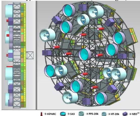
Fig.3 CAD design of gridded cluster plate including European electric thrusters with redundant PPUs for each thruster at the backside for the MARS/EUROPA-INPPS flagship.
