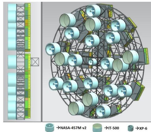
Fig. 6 CAD design of gridded cluster plate including Japanese, Russian and US electric thrusters with redundant PPUs for each thruster at the backside of the INPPS.
