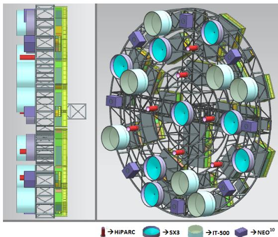
Fig. 5 CAD design of gridded cluster plate including European and Russian electric thrusters with redundant PPUs for each thruster at the backside. Thruster colours show the colour of the expected plume colour (depending on preferred propulsion).
