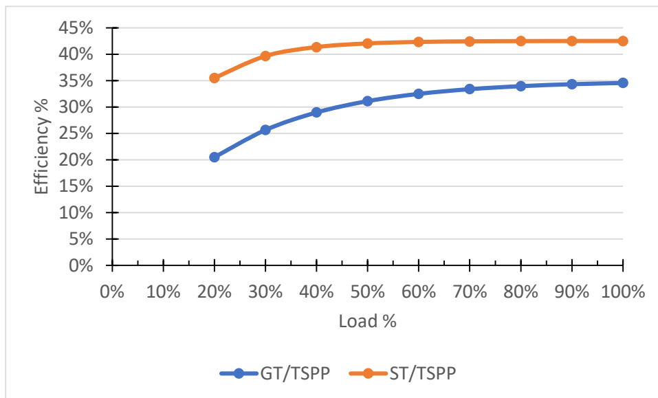
Figure 14: Efficiency of the TSPP's steam cycle (ST/TSPP) and gas turbine (GT/TSPP) as function of load. Below their minimum capacity of 20% the turbines are either shut down or kept at minimum power, in this case producing surplus.
