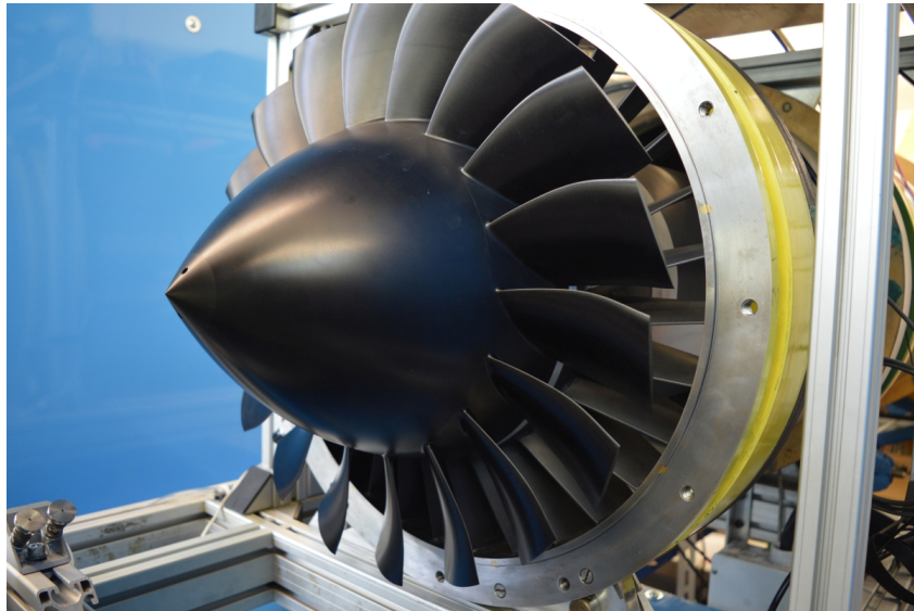
Figure 2.3: Implemented rotor without the casing
