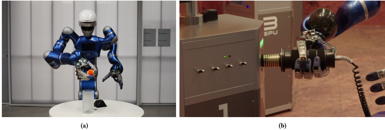
Figure 4: Evaluation scenarios. (a) Uncertain Environment: Rollin' Justin in front of a table with a tennis ball in hand about to drop it into a cylindrical container. (b) Insertion Action: Rollin' Justin in front of the SPU, about to connect the DIP to the SPU.
