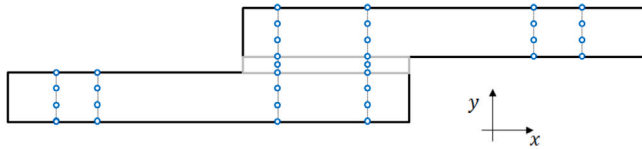
Fig. 8. Front view for coupling of displacement u_z applied on the nodes with the same x -coordinate belonging to the vertical lines on the edge. Source: Adopted from [38].
