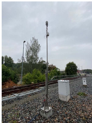
Figure 5: Example for a weather station: measuring system, here with additional noise component, the weather station at the top
