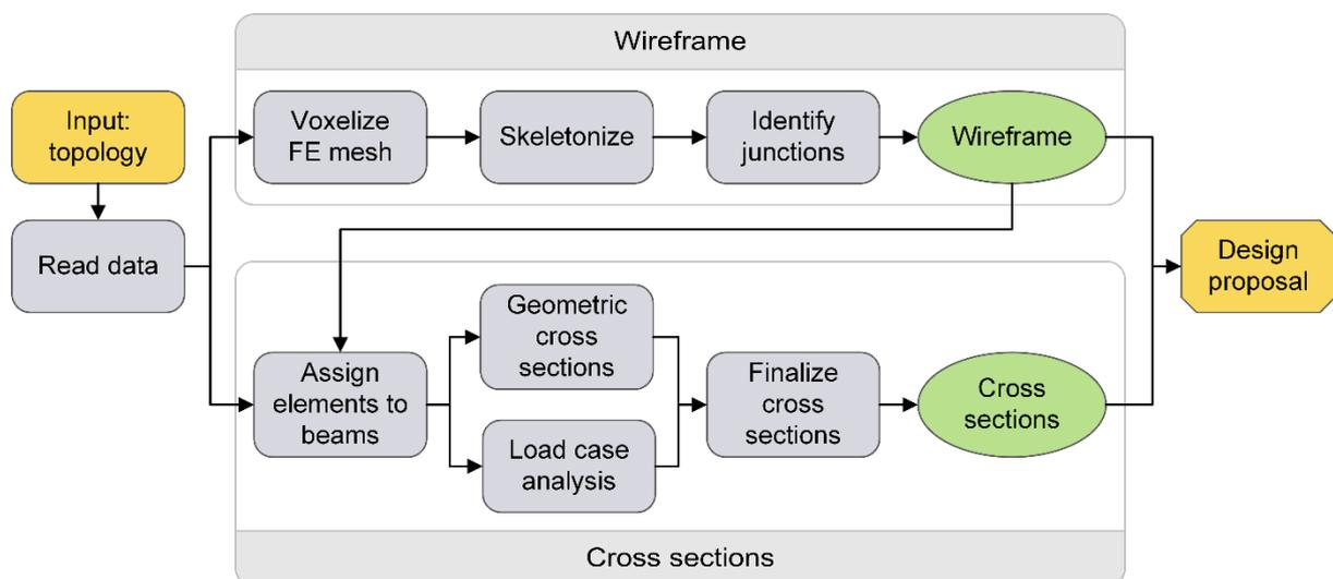
Figure 2: Automated process for deriving design proposals from topology optimizations
