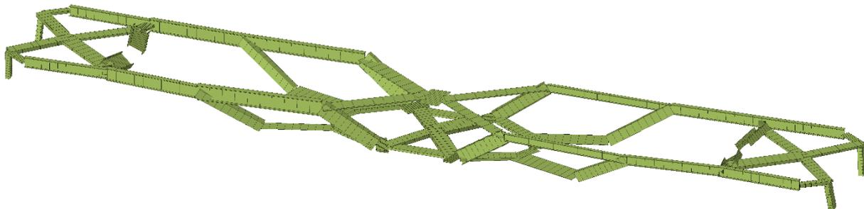
Figure 6: Automatically derived model using beam profiles in an FE application
