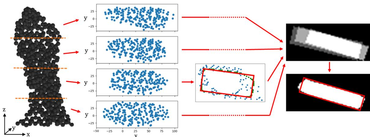
**Figure 4:** Geometric cross section analysis for beam consisting of a point cloud
