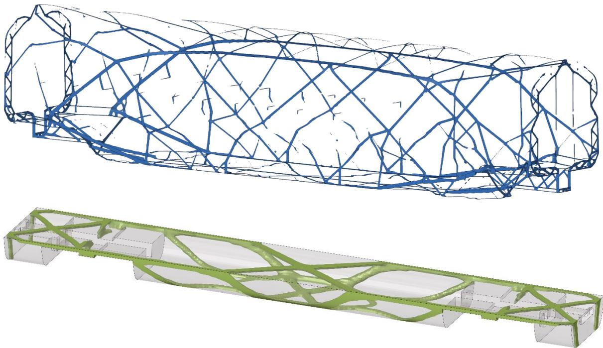
**Figure 1:** Topology optimization of the Aeroliner car body (top) and NGT CARGO undercarriage (bottom)
