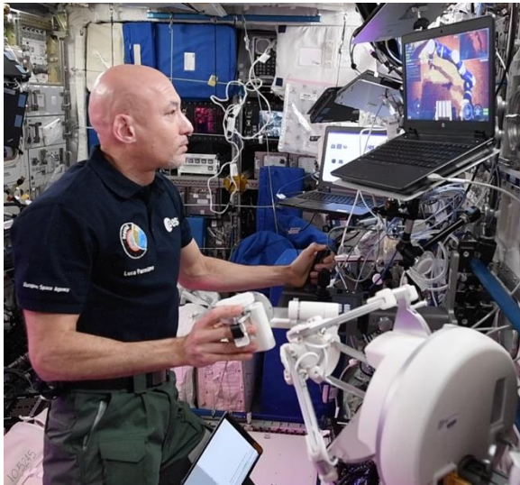
Figure 1. Luca Parmitano on the ISS controlling a rover on ground during ANALOG-1
