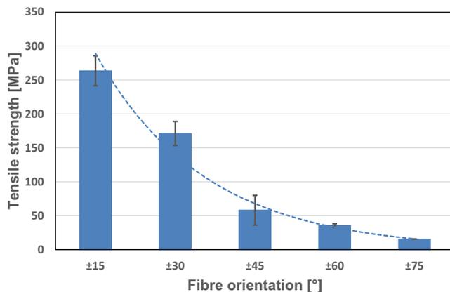
**FIGURE 4** Tensile strength versus fiber orientation at room temperature showing asymptotic behavior with trendline and standard deviation
