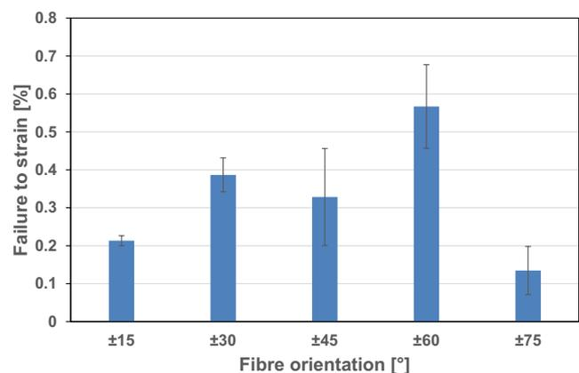
**FIGURE 5** Failure to strain versus fiber orientation at room temperature with standard deviation
