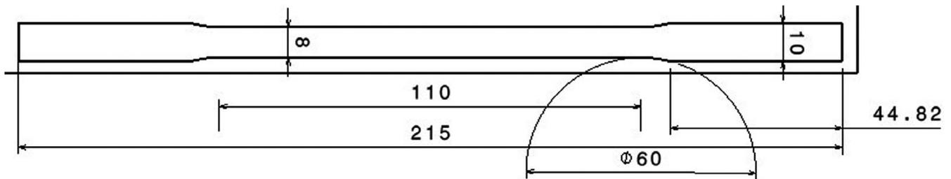
FIGURE 1 Specimen dimensions from C/C-SiC plates for tensile testing
