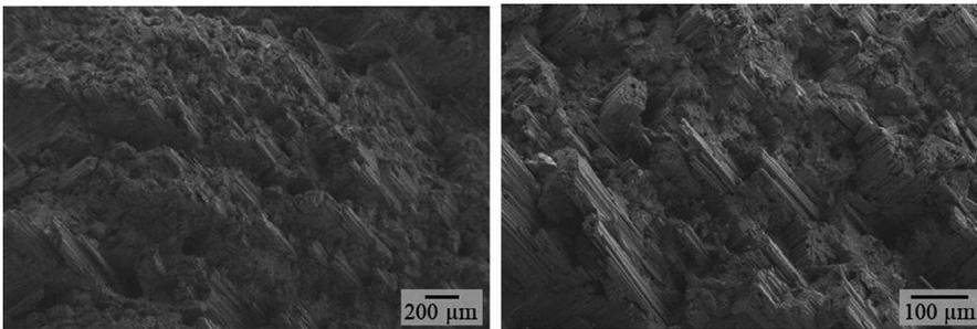
**FIGURE 15** Fracture surface of C/C-SiC with fiber orientation ±30° resembling a rather low fiber pull-out (magn. 100× [left] and 350× [right])
