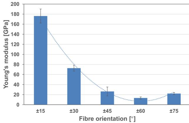
**FIGURE 6** Young's modulus versus fiber orientation at room temperature showing asymptotic behavior with trendline and standard deviation
