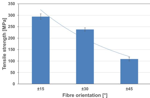
**FIGURE 10** Tensile strength versus fiber orientation at high temperature (1300°C) showing asymptotic behavior with trendline and standard deviation
