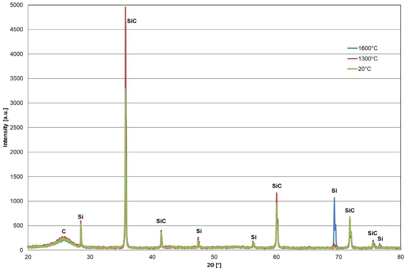
**FIGURE 25** XRD-diffractograms of C/C-SiC with fiber orientation  $\pm 45^\circ$  after being tested at  $1600^\circ\text{C}$  (blue),  $1300^\circ\text{C}$  (red), and original C/C-SiC (green) with same fiber orientation. Peak heights of C and SiC were kept constant, since their main amounts are predetermined by LSI processing and only the small amount of Si (typically in the range of 1%–2%) is sensitive to significant changes by gas phase processes
