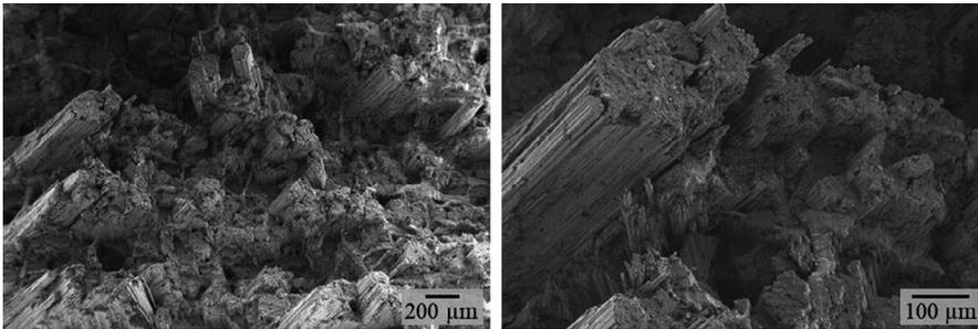
**FIGURE 14** Fracture surface of C/C-SiC with fiber orientation ±15° resembling a rather high fiber pull-out (magn. 100× [left] and 350× [right])
