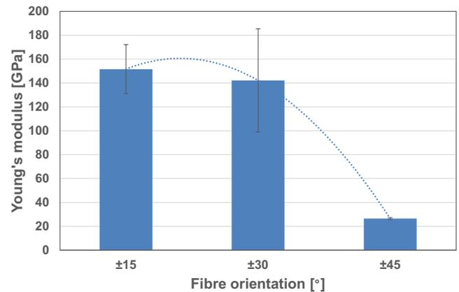
**FIGURE 12** Young's modulus versus fiber orientation at high temperature (1300°C) showing asymptotic behavior with trendline and standard deviation
