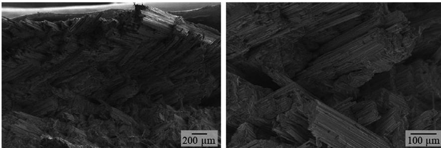
**FIGURE 16** Fracture surface of C/C-SiC with fiber orientation ±45° resembling fiber pull-out and matrix disintegration (magn. 100× [left] and 350× [right])
