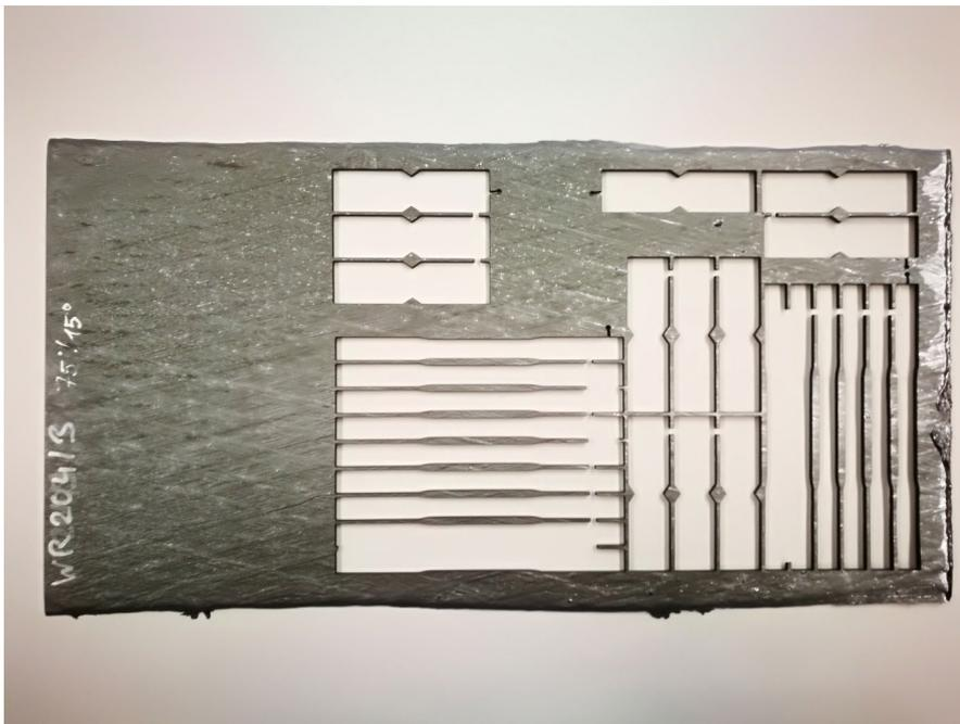
FIGURE 2 Preparation of specimens via jet-cutting from C/C-SiC plate with fiber orientation to tensile loading:  $\pm 15^\circ$  (horizontal) and  $\pm 75^\circ$  (vertical)
