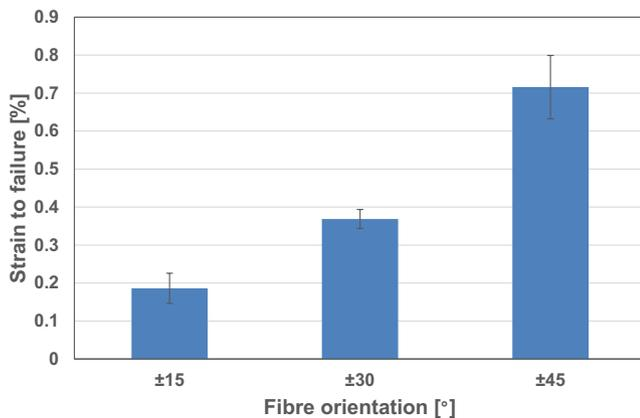
**FIGURE 11** Strain to failure versus fiber orientation at high temperature (1300°C) with trendline and standard deviation
