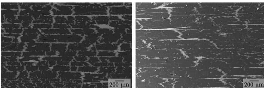
**FIGURE 9** Microstructure of C/C-SiC with fiber orientation ±60° (left) and ±75° (right)
