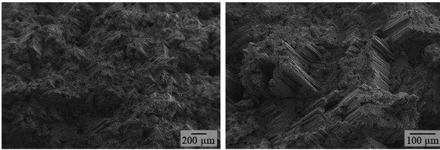
**FIGURE 20** Fracture surface of C/C-SiC with fiber orientation  $\pm 30^\circ$  after being tested at  $1,300^\circ\text{C}$  resembling a rather low fiber pull-out (magn.  $100\times$  [left] and  $350\times$  [right])
