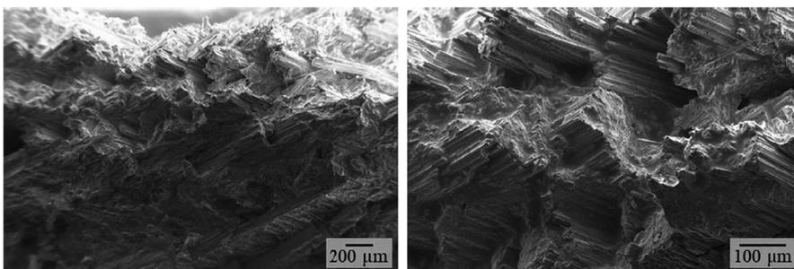
**FIGURE 23** Fracture surface of C/C-SiC with fiber orientation  $\pm 45^\circ$  after being tested at  $1,600^\circ\text{C}$  resembling a rather low fiber pull-out and rather brittle failure (magn.  $100\times$  [left] and  $350\times$  [right])
