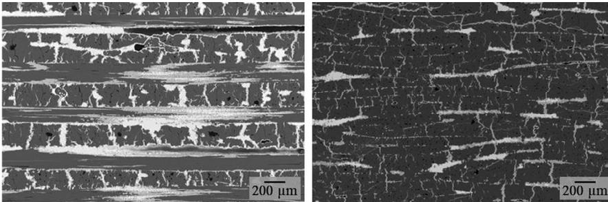
**FIGURE 7** Microstructure of C/C-SiC with fiber orientation 0°/90° (left) and ±15° (right)
