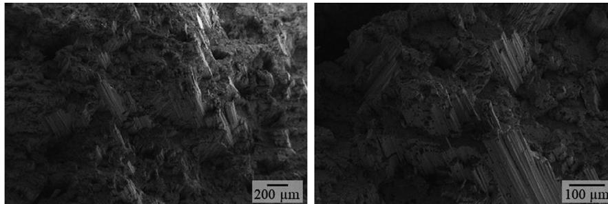
**FIGURE 19** Fracture surface of C/C-SiC with fiber orientation  $\pm 15^\circ$  after being tested at 1,300°C resembling a rather high fiber pull-out. But the amount of fiber pull-out seems to be slightly lower compared to the samples tested at room temperature (see Figure 14) (magn. 100 $\times$  [left] and 350 $\times$  [right])
