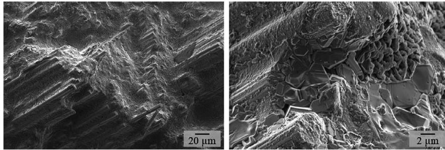
**FIGURE 24** Magnified fracture surface of C/C-SiC with fiber orientation  $\pm 45^\circ$  after being tested at  $1,600^\circ\text{C}$  resembling a rather low fiber pull-out and rather brittle failure. Note that C-fibers and C-matrix are covered with a thin structured coating, presumably SiC (magn.  $1,000\times$  [left] and  $10,000\times$  [right])
