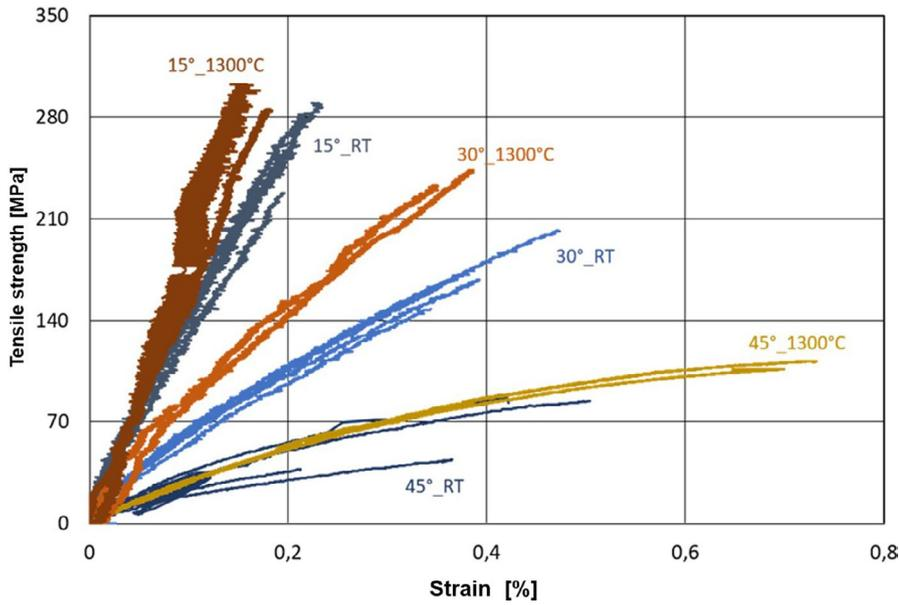
**FIGURE 13** Tensile behavior versus strain at room and high temperature (1300°C)
