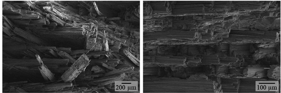
**FIGURE 18** Fracture surface of C/C-SiC with fiber orientation  $\pm 75^\circ$  resembling high amount of matrix disintegration; almost no matrix is visible anymore (magn. 100 $\times$  [left] and 350 $\times$  [right])
