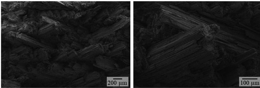
**FIGURE 21** Fracture surface of C/C-SiC with fiber orientation  $\pm 45^\circ$  after being tested at  $1,300^\circ\text{C}$  resembling a rather low fiber pull-out and matrix disintegration; almost no matrix is visible anymore (magn.  $100\times$  [left] and  $350\times$  [right])
