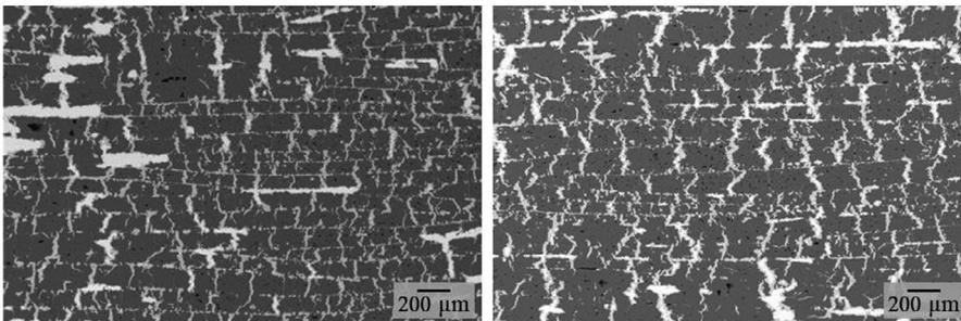
**FIGURE 8** Microstructure of C/C-SiC with fiber orientation ±30° (left) and ±45° (right)
