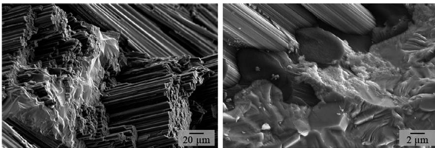
**FIGURE 22** Magnified fracture surface of C/C-SiC with fiber orientation  $\pm 45^\circ$  after being tested at  $1,300^\circ\text{C}$  resembling a rather low fiber pull-out and matrix disintegration; no coating is visible (magn.  $1,000\times$  [left] and  $10,000\times$  [right])
