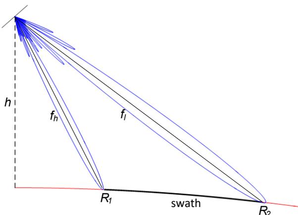
Figure 3 Active phased array antenna at altitude  $h$ . Highest frequency  $f_h$ , lowest frequency  $f_l$ .
