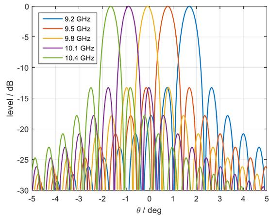
Figure 4 Antenna pattern for dispersive elevation beam.
