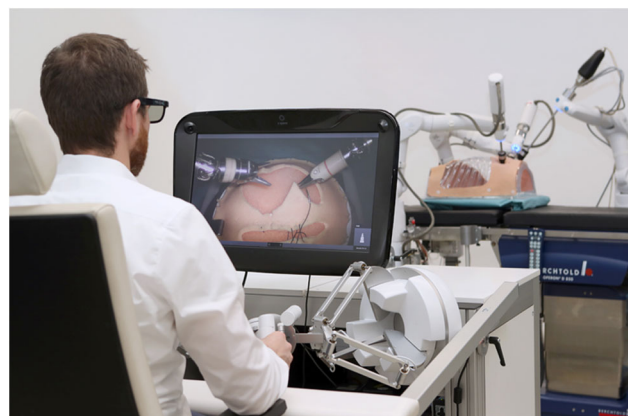
Fig. 6 MiroSurge—The DLR research platform for telemanipulation in minimally invasive robotic surgery (Alexandra Beier/DLR CC-BY 3.0)
