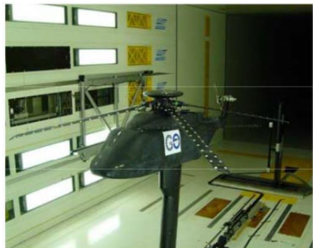
Figure 1: 7AD rotor in the GOAHEAD setup.
